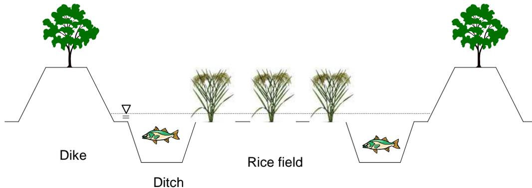
Figure 1. Transect of a typical rice–fish plot in the Mekong delta: a rice field, ditches as a refuge for fish when water is low and, to keep the fish inside, a peripheral dike with vegetables or fruit trees.
