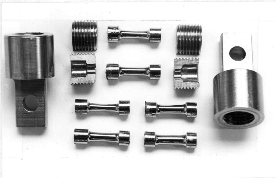
(a) Some single crystal tensile specimens and grips
