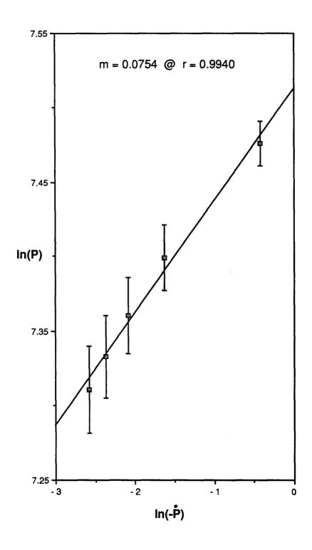
Figure 16. Strain rate sensitivity index for PVC derived from stress relaxation testing average parameter data.
