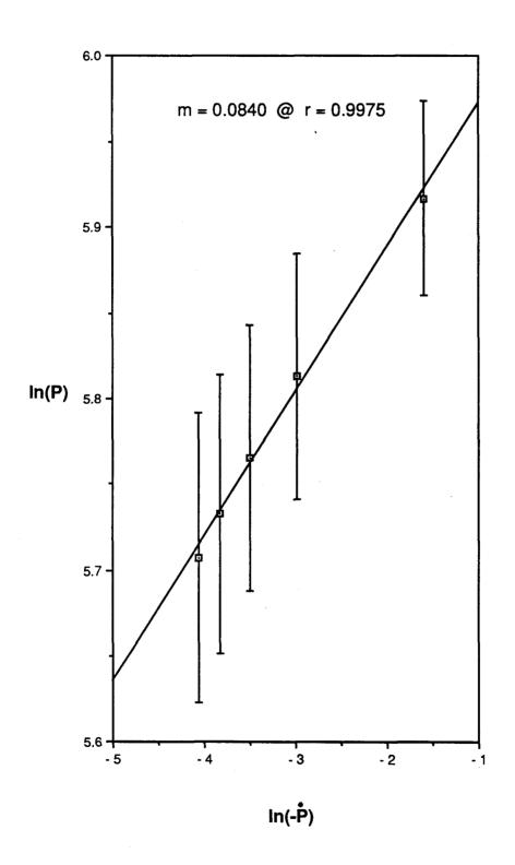
Figure 15. Strain rate sensitivity index for PA derived from stress relaxation testing average parameter data.
