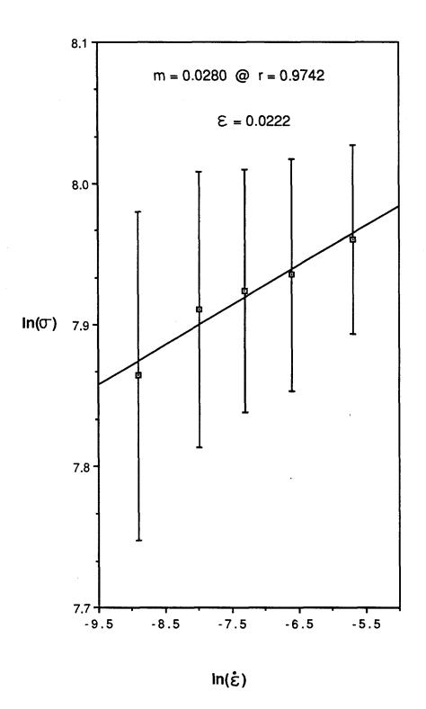
Figure 6. Strain rate sensitivity index for PVC derived from variable strain rate testing average modulus and strain data.
