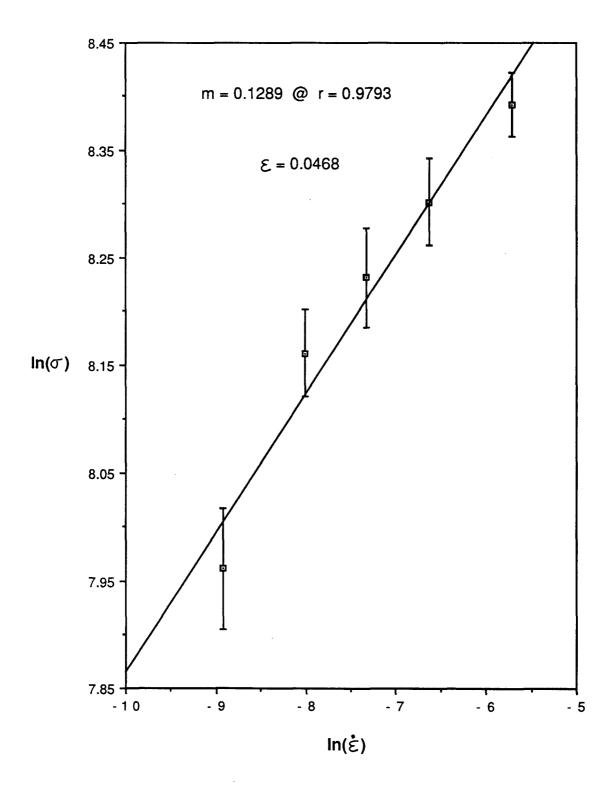
Figure 3. Strain rate sensitivity index for PP derived from variable strain rate testing average modulus and strain data.
