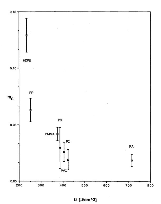
Figure 20. Strain rate sensitivity index derived from stress relaxation testing as a function of cohesive energy density.
