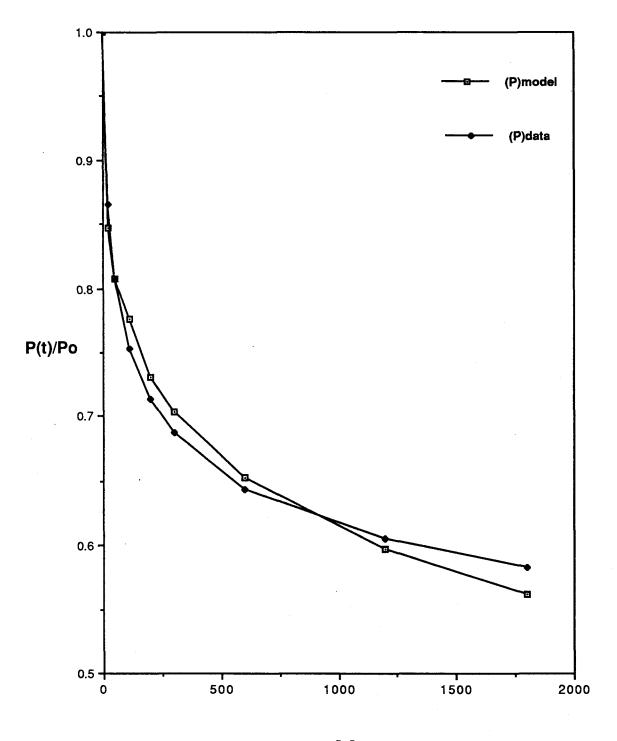
Figure 10. Normalized relaxation response for PC, PMMA, PA, PVC, PP, PS, and HDPE derived from average parameter data.
