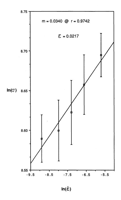
Figure 5. Strain rate sensitivity index for PS derived from variable strain rate testing average modulus and strain data.
