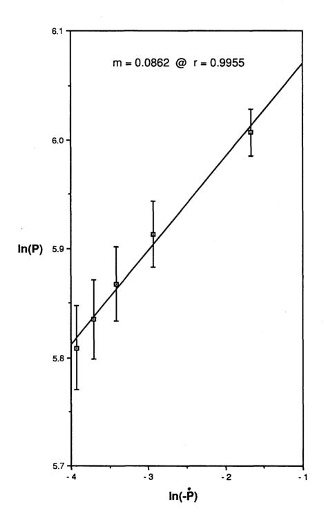
Figure 14. Strain rate sensitivity index for PS derived from stress relaxation testing average parameter data.
