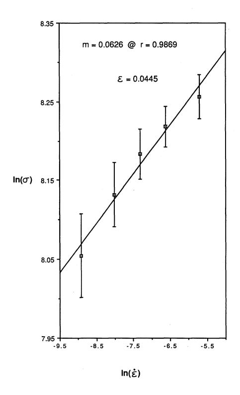
Figure 4. Strain rate sensitivity index for PMMA derived from variable strain rate testing average modulus and strain data.
