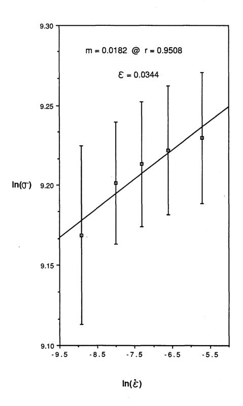
Figure 8. Strain rate sensitivity index for PC derived from variable strain rate testing average modulus and strain data.
