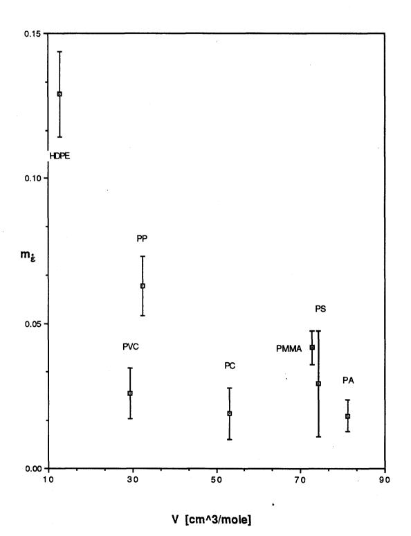
Figure 22. Strain rate sensitivity index derived from stress relaxation testing as a function of molar volume.
