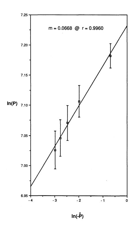
Figure 17. Strain rate sensitivity index for PC derived from stress relaxation testing average parameter data.
