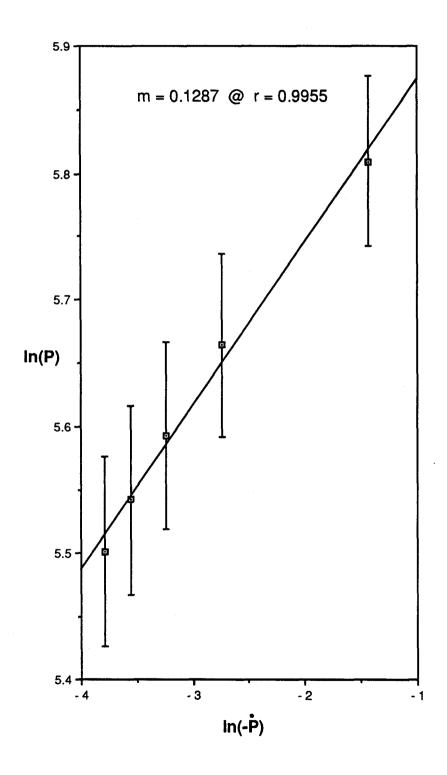
Figure 13. Strain rate sensitivity index for PP derived from stress relaxation testing average parameter data.
