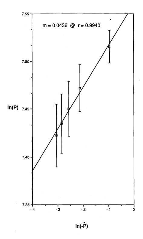
Figure 18. Strain rate sensitivity index for PMMA derived from stress relaxation testing average parameter data.
