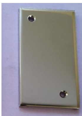
Figure 24. Photograph of corona micro reactor counter electrode
