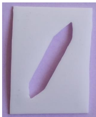
Figure 23. Photograph of corona microreactor channel geometry
