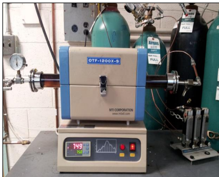
Figure 19. Photograph OTF 1200X-S split tube furnace with 2" O.D quartz tube CVD from MTI Corporation experiment
