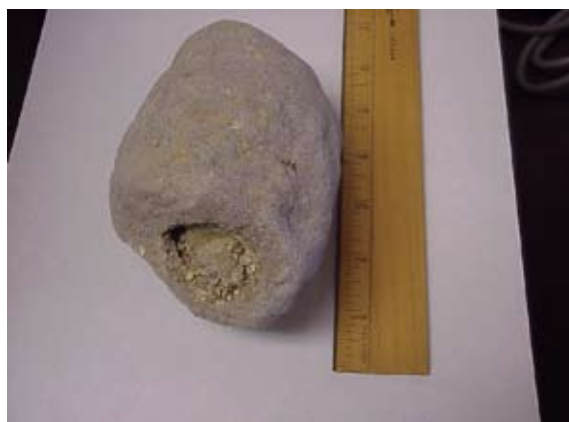
Figure 8.—A large, cemented clod of soil taken from an apple orchard in eastern Washington. Before the center of the clod was treated with elemental sulfur and N-phuric, the soil pH was 8.9. After S application, the soil pH at the clod surface was 2.5, thus demonstrating how small, localized changes can impact pH.
