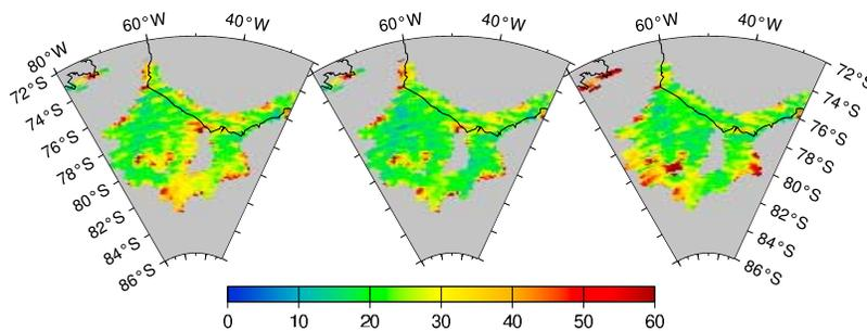
**Figure 3.** Mean ICESat crossover discrepancies (cm) over the Filchner and Ronne Ice Shelves as function of adopted tide model: (left) TPXO7.1, (middle) this paper, (right) FES2004. Corresponding RMS statistics for this region are tabulated in Table 2.
