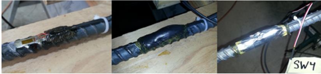
Fig. 3.17 – Application of strain gage on reinforcing bar
