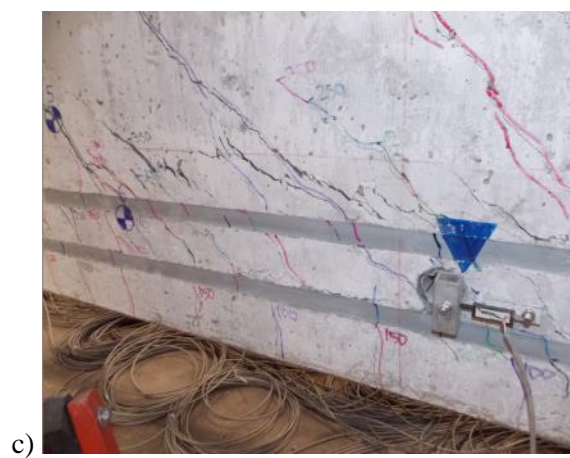
Fig. 4.4 - Specimen T.45.Ld3(6).Ti at failure; a) front, b) back, c) detail of cutoff bar slip
