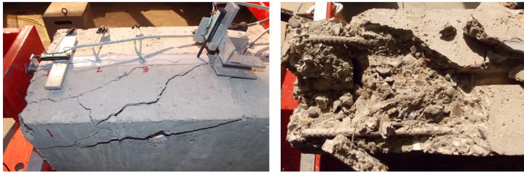
Fig. 4.38 - 12 in. bond length specimen at failure (left) and detail of remaining concrete (right)
