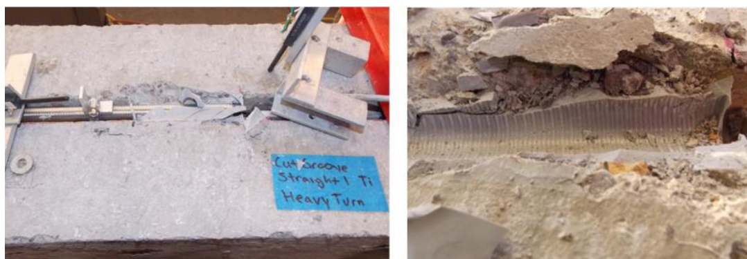
Fig. 4.34 – Bond length specimen at failure (left) and detail of failure (right)
