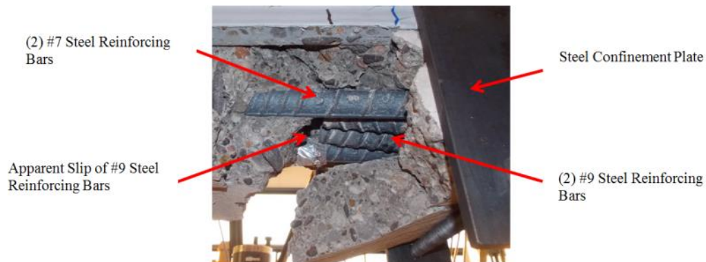
Fig. I.27 - Apparent slip of #9 Steel Reinforcing Bars in Mosier 3
