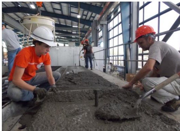
Fig. 3.11 - Typical construction of T-specimen
