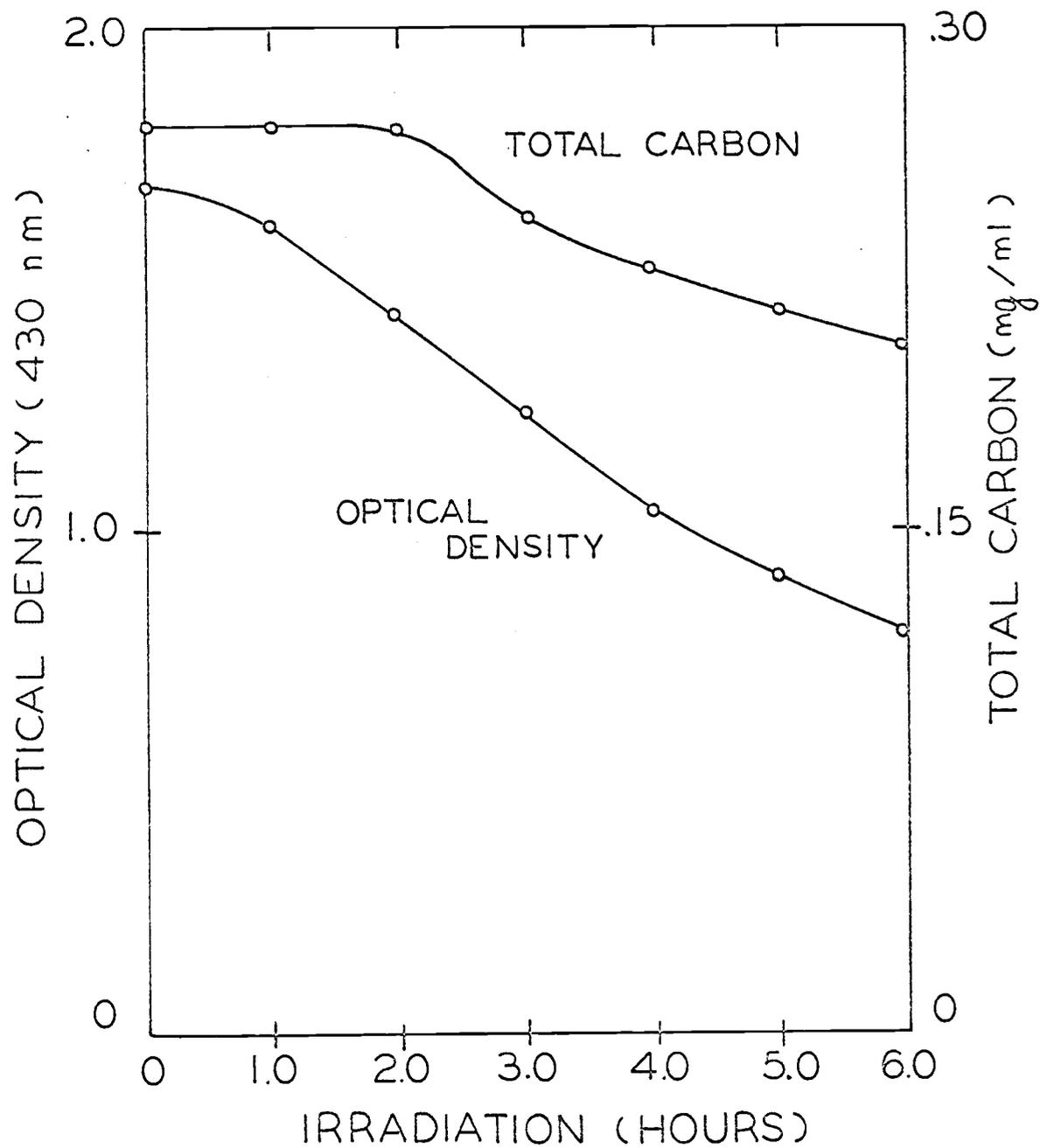
Figure 4. Effects of wavelengths longer than 210.0 nm on decoloration and total carbon of 0.05% w/v sodium ligninsulfonate solution
