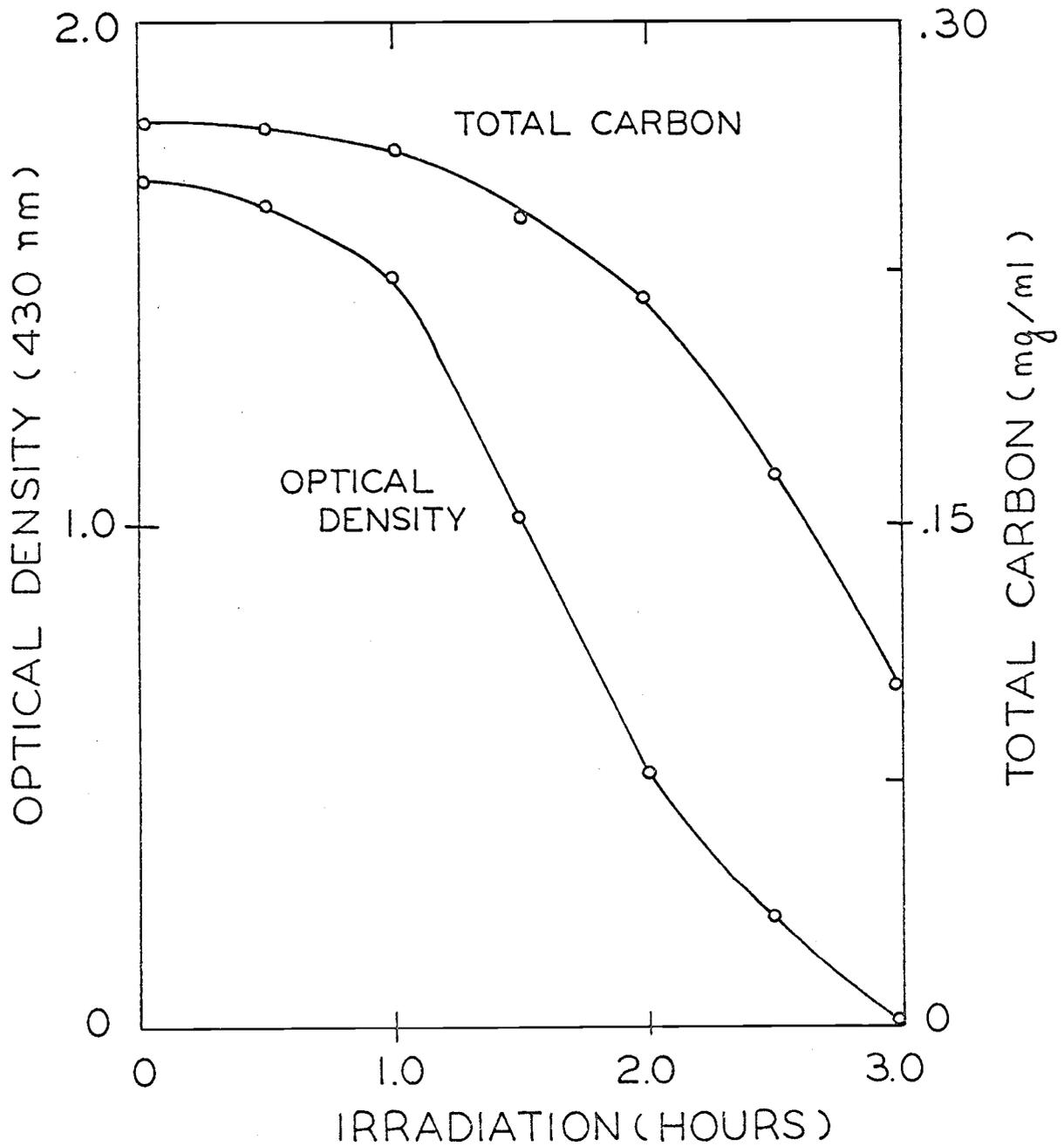
Figure 5. Effects of wavelengths longer than 184.9 nm on decoloration and total carbon of 0.05 w/v sodium ligninsulfonate solution
