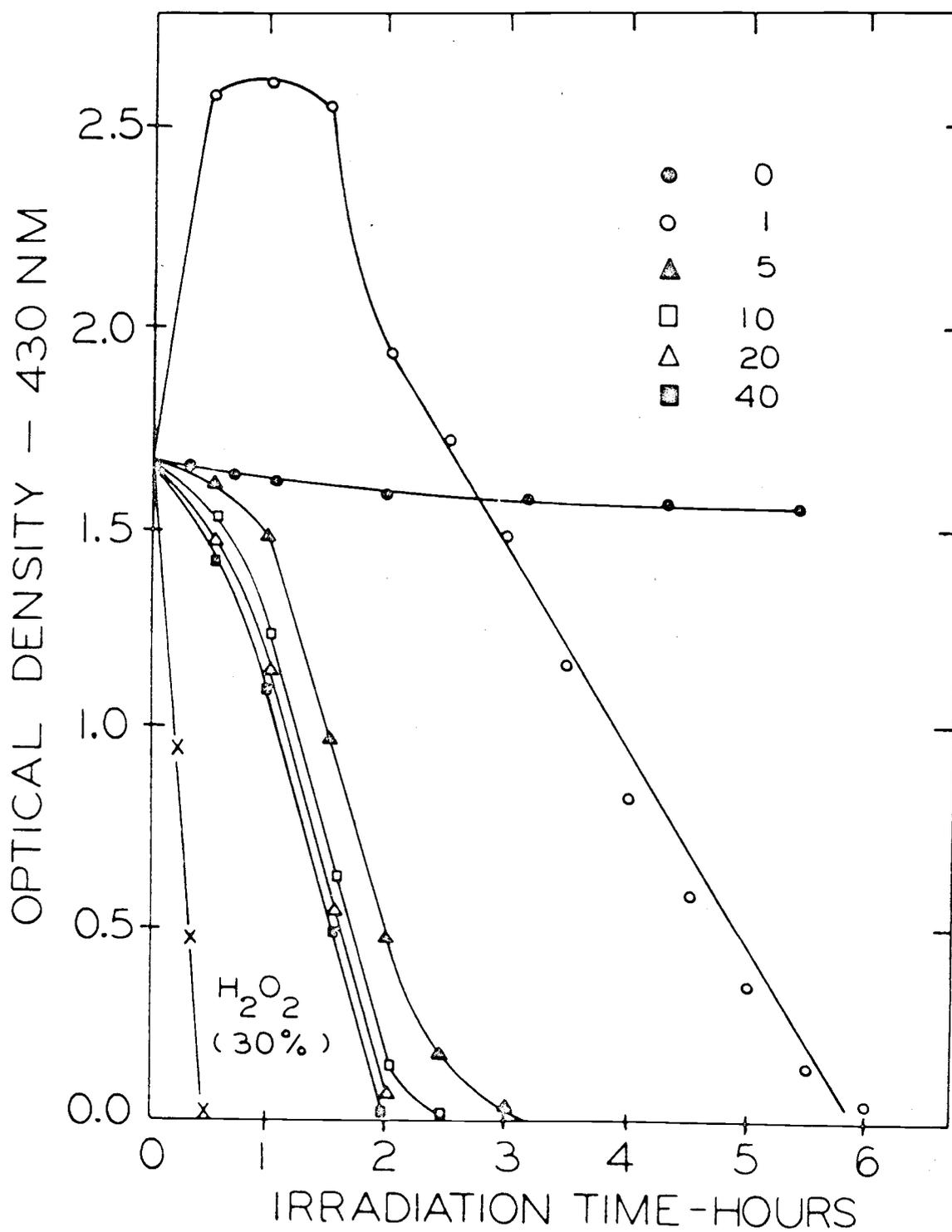
Figure 1. Effect of oxygen flow rate (ml/min) on decoloration of 0.05 w/v sodium ligninsulfonate solution
