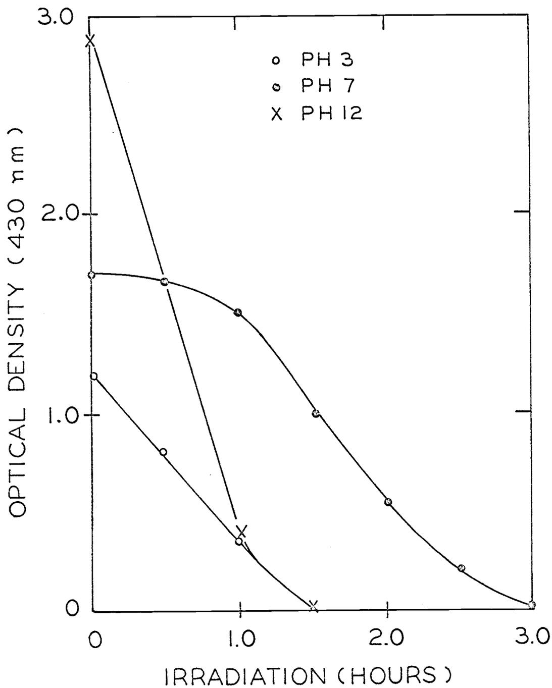
Figure 2. Effect of initial pH on decoloration of 0.05% w/v sodium ligninsulfonate
