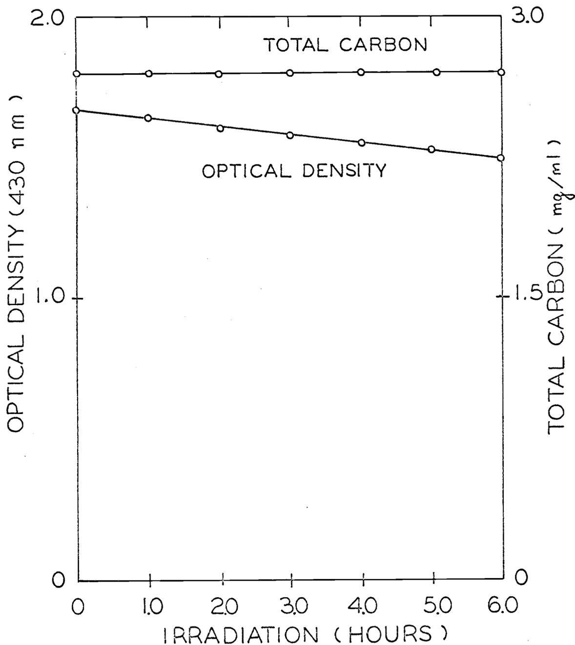
Figure 3. Effects of wavelengths longer than 280.0 nm on decoloration and total carbon of 0.05% w/v sodium ligninsulfonate solution
