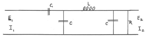
The resistance of the short circuit is considered for the purpose of analysis, but for the final equation, R is placed equal to zero.
