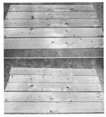
Figure 2. Planks in charge 5 (top), with initial conditions for 12 per cent Emc, checked more and were 15 hours longer in kiln than charge 5A (below),
