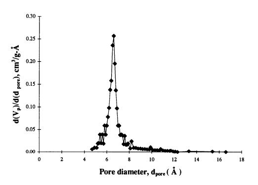
Figure 4. Pore size distribution of HY-zeolite.
