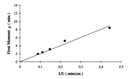
Figure 17. First moment of glucose diffusion in packed column of HY-zeolite catalyst (trial # 1).
