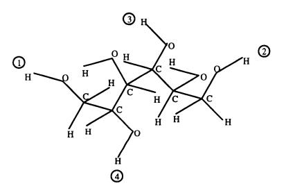
The length between (1) and (2) is equal to 7.31422 Å, and the length between (3) and (4) is equal to 5.60102 Å ( calculated by Hyperchem Software ). The long axis is the
