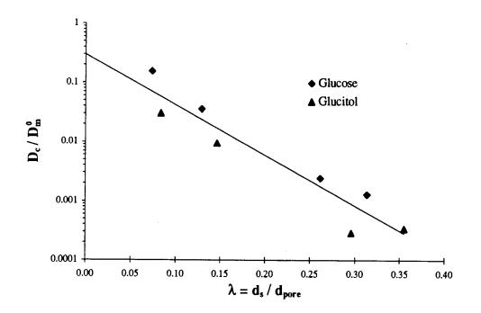
Figure 38. Effect of  $\lambda$  on the intracrystalline diffusivity (D<sub>c</sub>).
