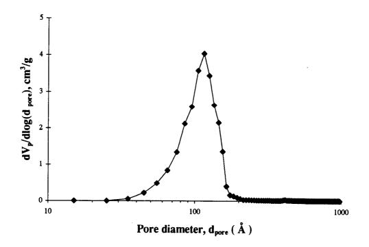
Figure 8. Pore size distribution of silica gel-100.
