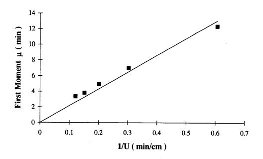
Figure 18. First moment of glucose diffusion in packed column of Na-MCM-20 catalyst (trial # 1).
