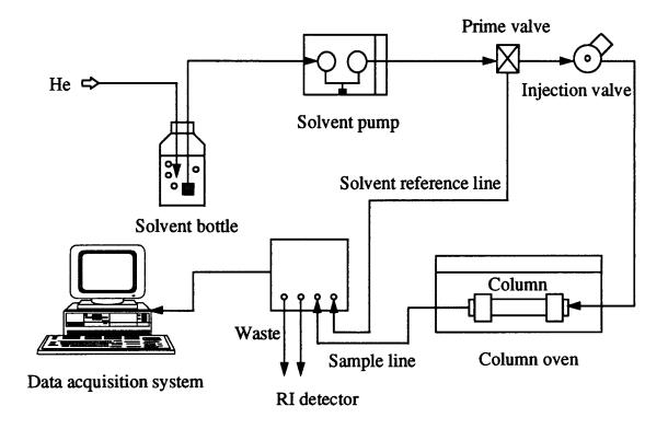
Figure 14. High Performance Liquid Chromatography (HPLC) system.
