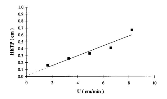
Figure 28. HETP of glucose diffusion in packed column of Na-MCM-20 catalyst (trial # 1).
