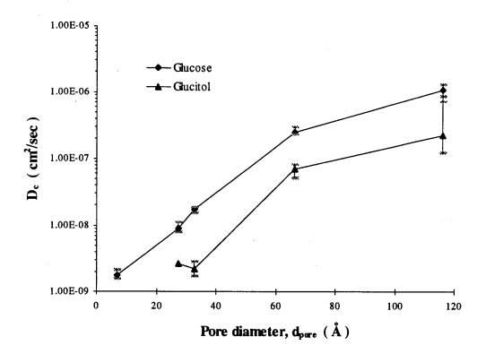
Figure 37. Effect of the pore size  $(d_{pore})$  on the intracrystalline diffusivity  $(D_c)$ .
