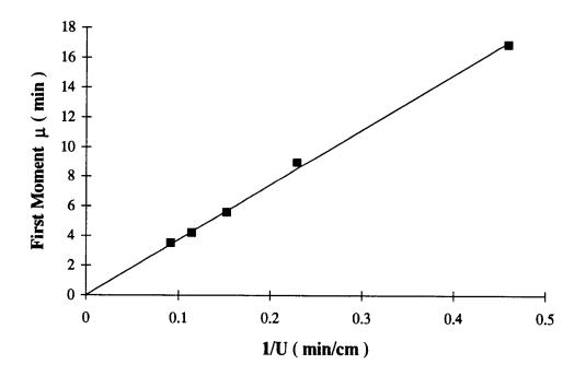
Figure 25. First moment of glucitol diffusion in packed column of silica gel-60 catalyst (trial # 1).
