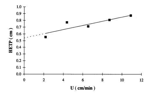
Figure 35. HETP of glucitol diffusion in packed column of silica gel-60 catalyst (trial # 1).
