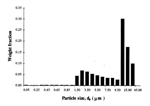
Figure 11. Particle size distribution of Na-MCM-41.
