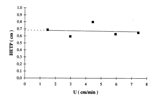
Figure 32. HETP of glucitol diffusion in packed column of HY-zeolite catalyst (trial # 1).
