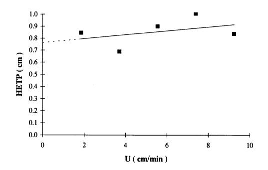
Figure 36. HETP of glucitol diffusion in packed column of silica gel-100 catalyst (trial # 1).
