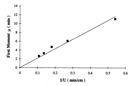
Figure 21. First moment of glucose diffusion in packed column of silica gel-100 catalyst (trial # 1).
