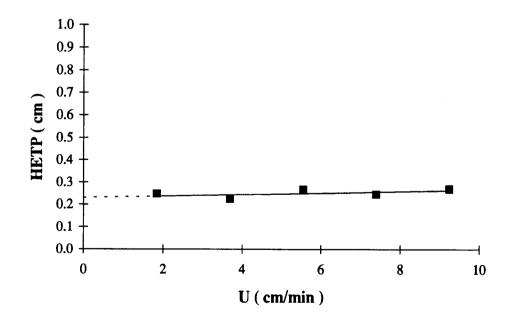
Figure 31. HETP of glucose diffusion in packed column of silica gel-100 catalyst (trial # 1).
