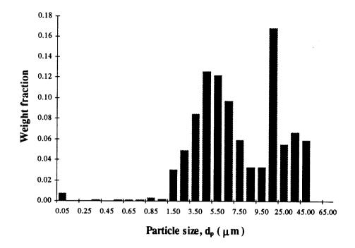
Figure 9. Particle size distribution of HY-zeolite.
