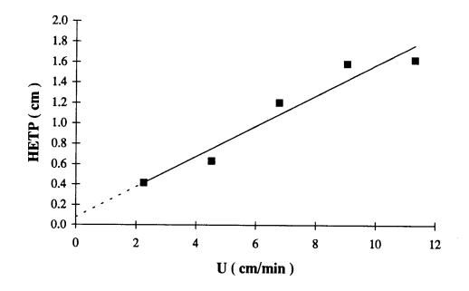
Figure 27. HETP of glucose diffusion in packed column of HY-zeolite catalyst (trial # 1).
