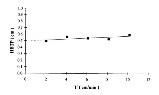
Figure 30. HETP of glucose diffusion in packed column of silica gel-60 catalyst (trial # 1).
