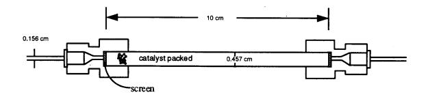
Figure 15. Schematic packed catalyst column.
