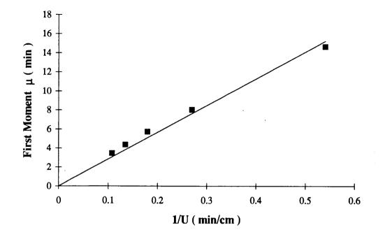
Figure 26. First moment of glucitol diffusion in packed column of silica gel-100 catalyst (trial # 1).
