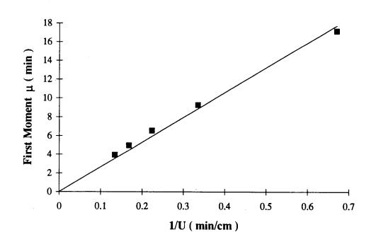
Figure 22. First moment of glucitol diffusion in packed column of HY-zeolite catalyst (trial # 1).
