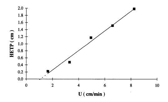
Figure 33. HETP of glucitol diffusion in packed column of Na-MCM-20 catalyst (trial # 1).
