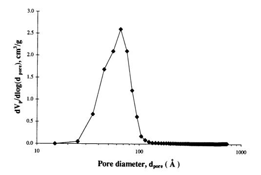
Figure 7. Pore size distribution of silica gel-60.
