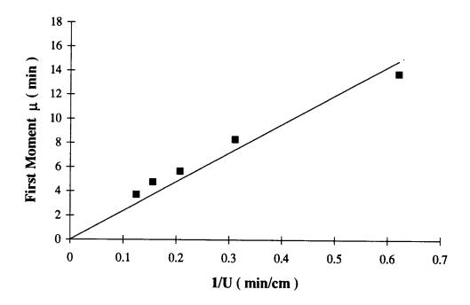
Figure 24. First moment of glucitol diffusion in packed column of Na-MCM-41 catalyst (trial # 1).
