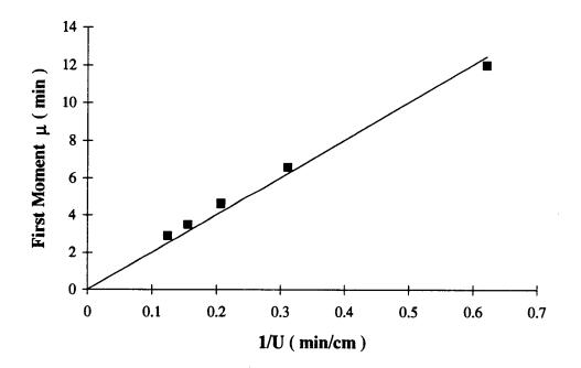
Figure 19. First Moment of glucose diffusion in packed column of Na-MCM-41 catalyst (trial # 1).
