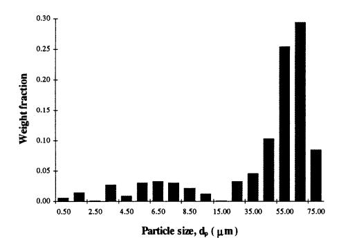
Figure 12. Particle size distribution of silica gel-60.
