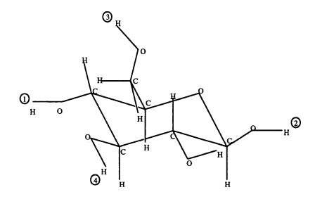
The length between (1) and (2) is equal to 6.01724 Å, and the length between (3) and (4) is equal to 6.18282 Å ( calculated by Hyperchem Software ). The longest short axis is the length between (1) and (2) including the radius of H, and the long axis is the length between (3) and (4) including the radius of H.
