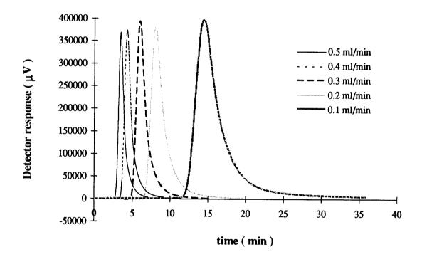
Figure 16. Response peaks of glucose diffusion in packed column of silica gel-100 catalyst (trial # 1).
