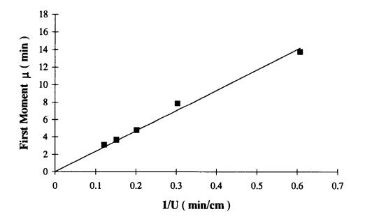
Figure 23. First moment of glucitol diffusion in packed column of Na-MCM-20 catalyst (trial # 1).
