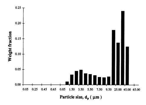
Figure 10. Particle size distribution of Na-MCM-20.
