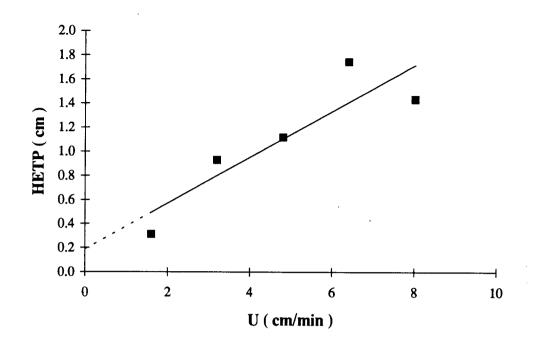
Figure 34. HETP of glucitol diffusion in packed column of Na-MCM-41 catalyst (trial # 1).
