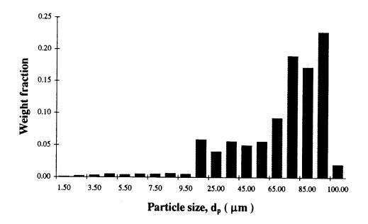
Figure 13. Particle size distribution of silica gel-100.
