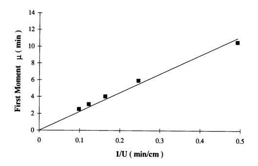
Figure 20. First moment of glucose diffusion in packed column of silica gel-60 catalyst (trial # 1).
