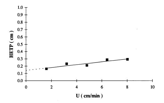
Figure 29. HETP of glucose diffusion in packed column of Na-MCM-41 catalyst (trial # 1).
