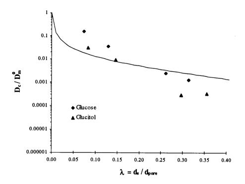
Figure 39. Diffusivity of solute vs.  $\lambda$  based on Ternan's model.
