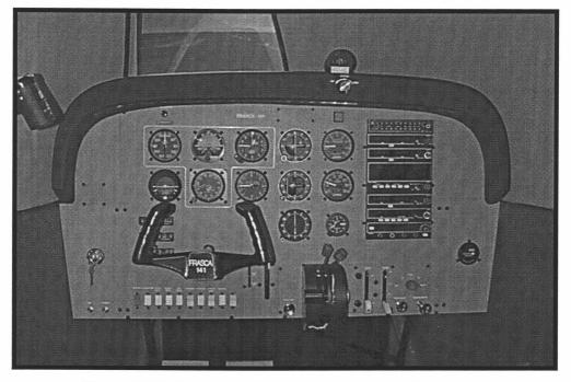
Figure 2.8 The Frasca 141 Instrument Displays and Controls.
