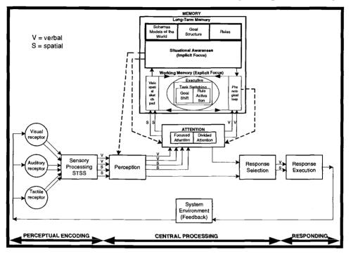
Figure 2.4 The Augmented Stage Model of Human-Information Processing.
