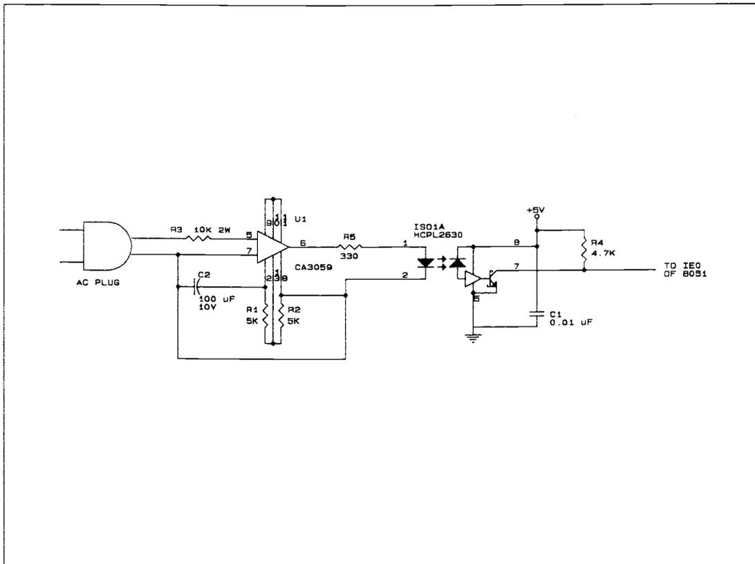
Figure 4-4. Zero-Crossing Detect Circuitry.
