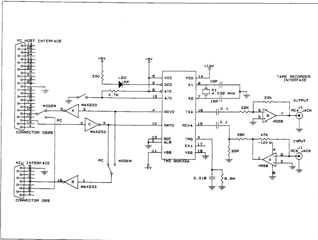
Figure 4-7. Modem Utilizing the TMS 99532A.
