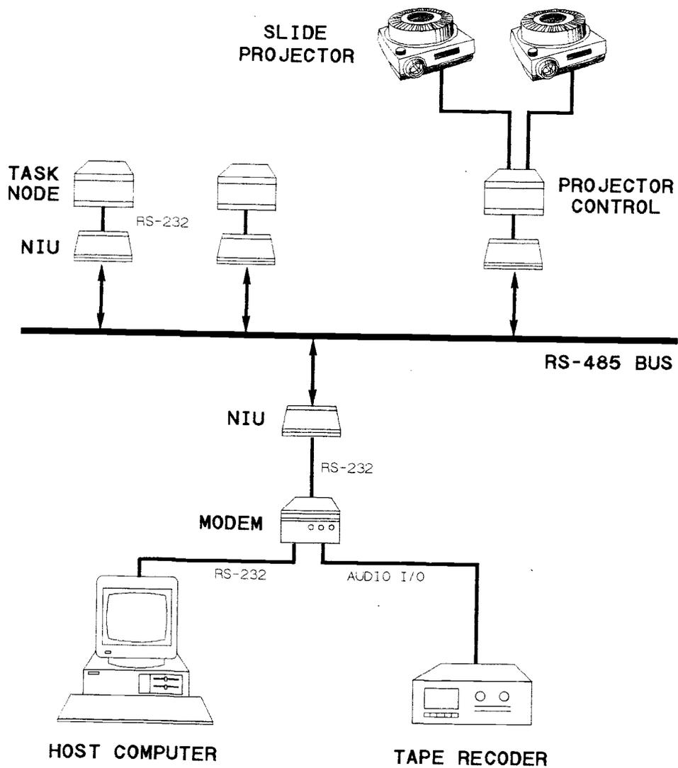
Figure 1-1. COLAN V - Multi-Media Network Configuration.
