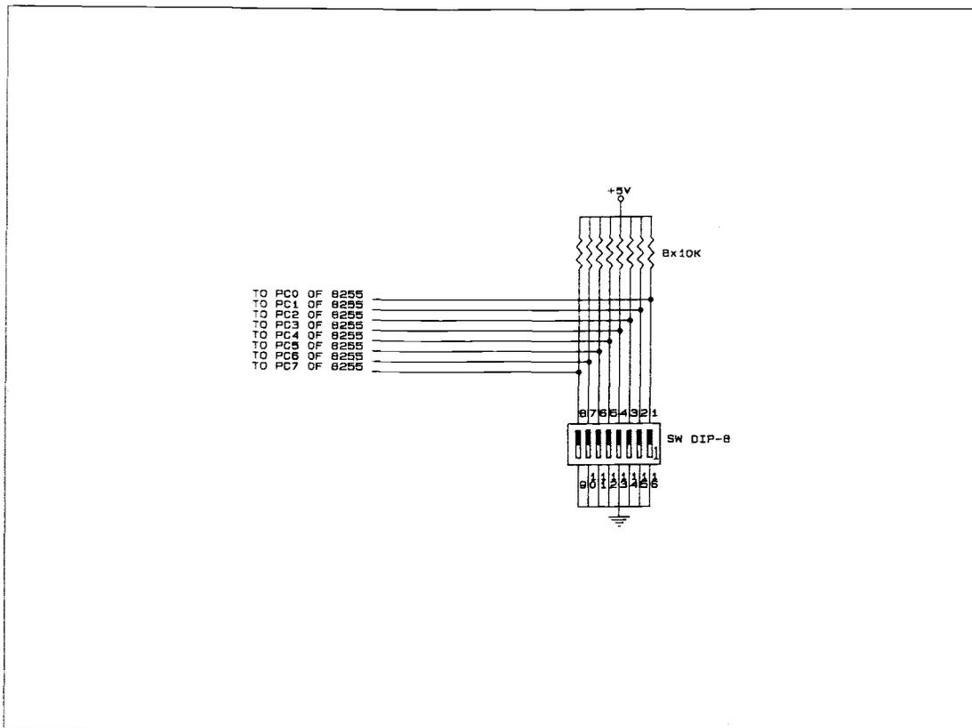
Figure 4-9. Node Address and Baud Rate Select Circuitry.
