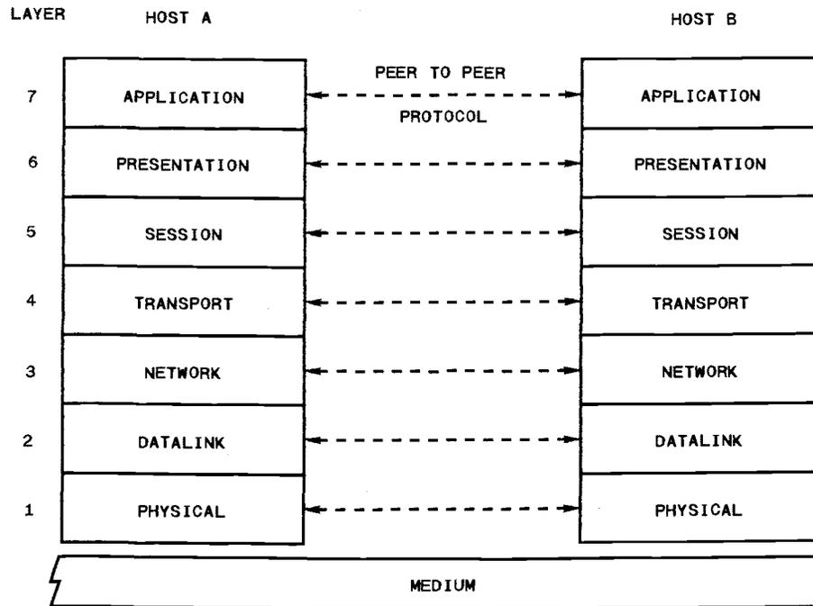
Figure 2-2. ISO Open System Interconnect Model [MYER 82].
