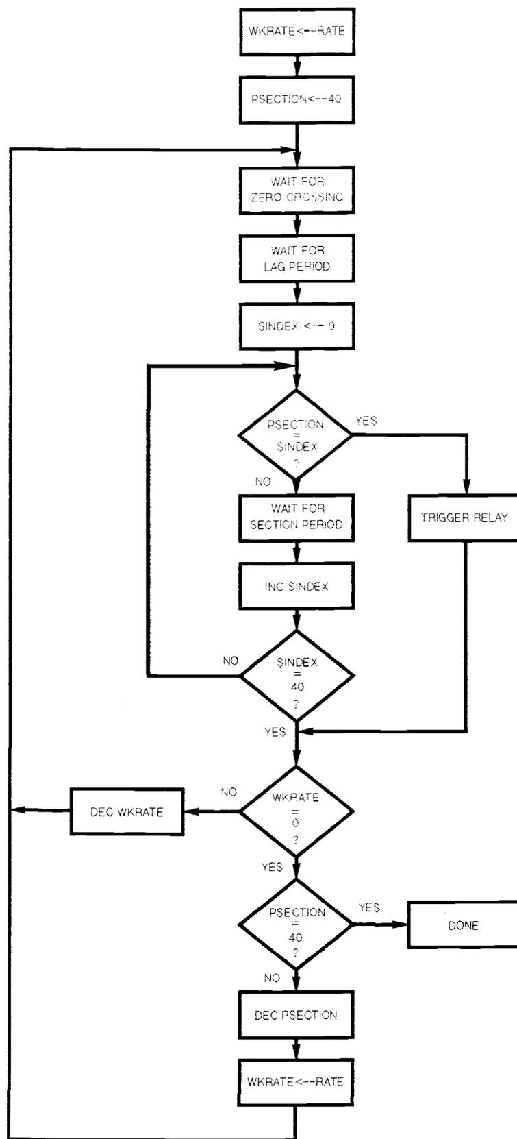
Figure 5-3. Flowchart for Bring a Lamp to Full Brightness.
