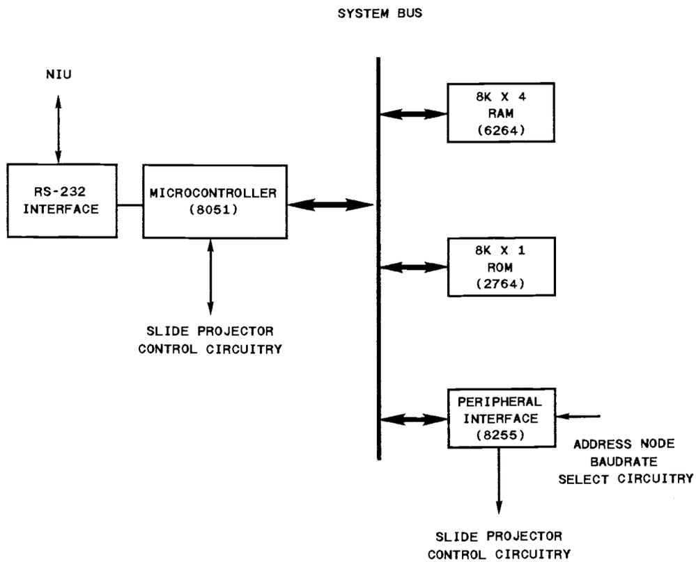
Figure 4-2. Microcontroller-Based System.
