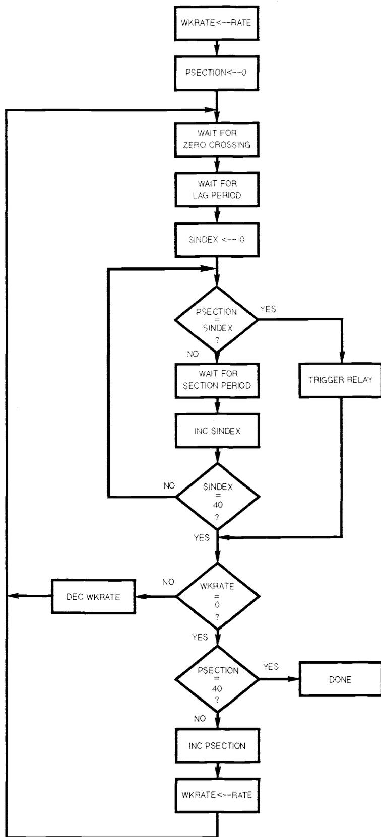
Figure 5-2. Flowchart for Dimming a Lamp.
