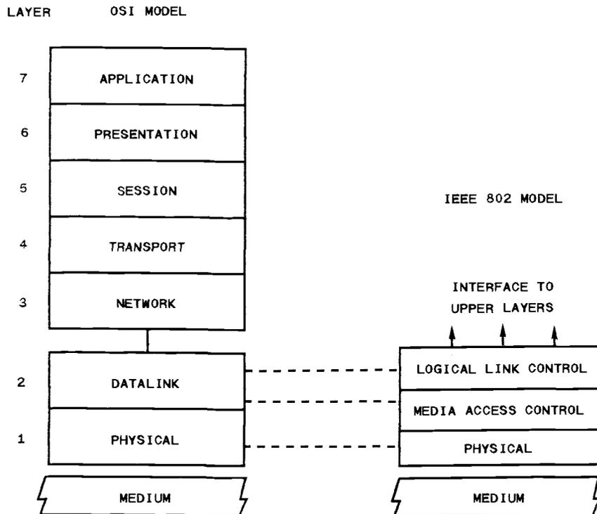
Figure 2-3. IEEE 802 Model Relationship to OSI Model [STAL 84].
