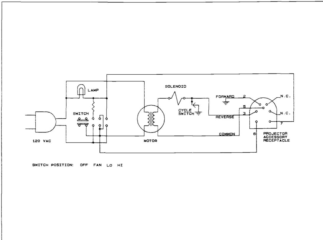
Figure 4-5. Slide Projector Internal Control Circuitry.
