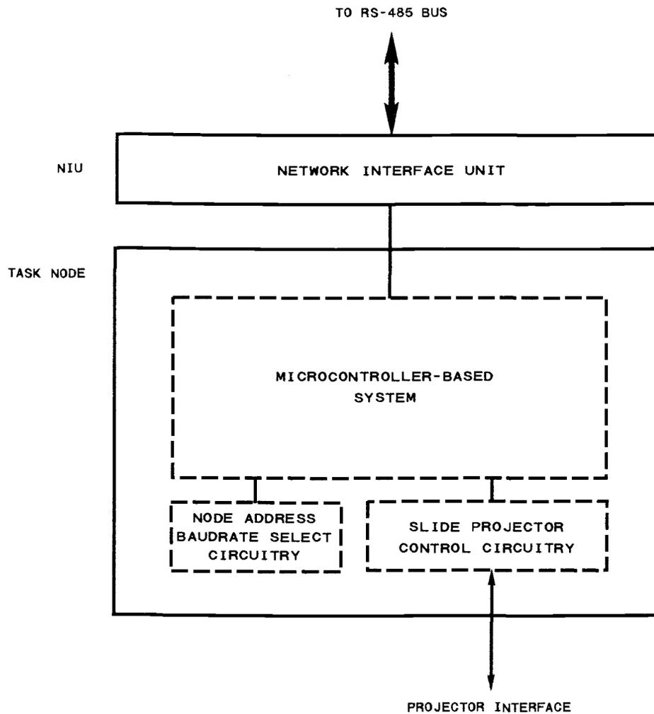
Figure 4-1. Task Node to Network Bus Interface.
