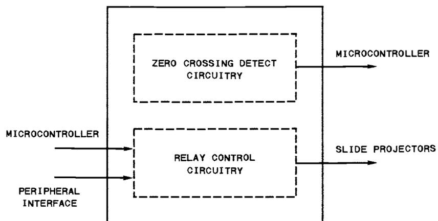
Figure 4-3. Slide Projector Control Circuitry.
