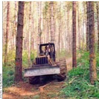
Figure 3.—Harvesting with a rubber-tire skidder.
