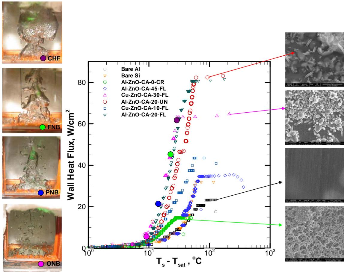
Figure 5: Pool boiling curves for nano-textured surfaces compared against bare Al and Si surfaces. Visual images of various pool boiling stages are highlighted on the left and their corresponding locations are highlighted as filled circles on Cu-30 Contact Angle boiling curve (ONB – Onset of Nucleate Boiling ⇒ PNB – Partial Nucleate Boiling ⇒ FNB – Fully-Developed Nucleate Boiling ⇒ CHF – Critical Heat Flux).
