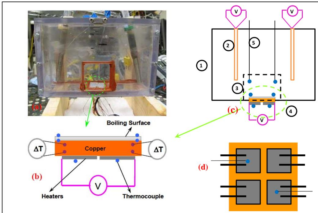
Figure 3: (a) Boiling test facility for pool-boiling performance characterization, (b) schematic illustration of the instrumented test heater set-up (filled blue circles are implemented thermocouples), (c) schematic of the boiling set-up (1: boiling chamber, 2: immersion heater, 3: visual window, 4: heating block, 5: thermocouple), and (d) schematic of the heater assembly.
