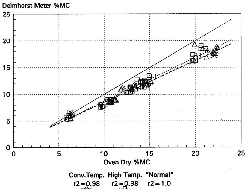
Figure 4. Data and regression lines for norway spruce tested with a resistance-type meter and 21% while the conventionally dried wood equilibrated to 11 and 22%. This did not, however, affect meter accuracy.
