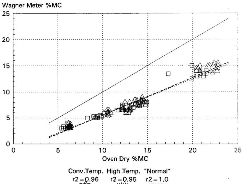
Figure 5. Data and regression lines for red pine tested with a capacitance-type meter.
