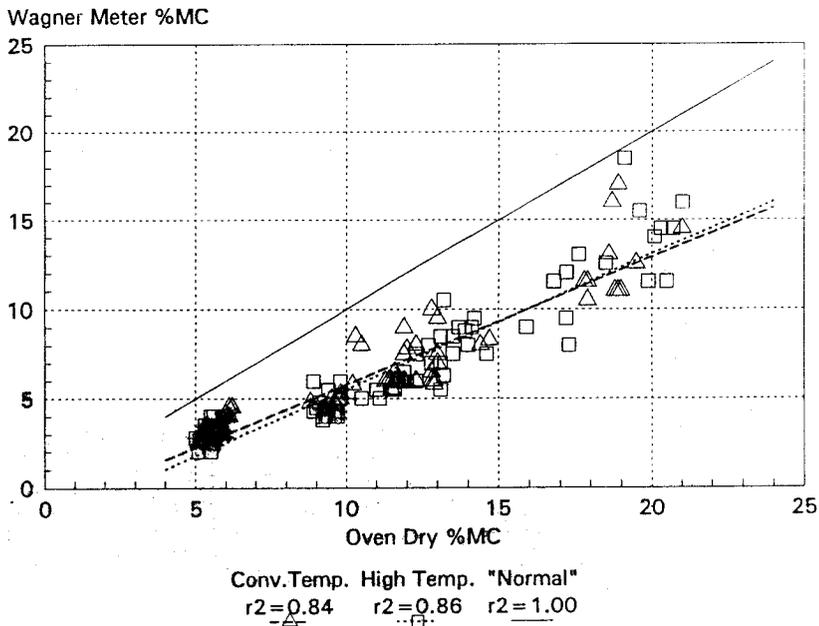
Figure 6. Data and regression lines for eastern white pine tested with a capacitance-type meter.
