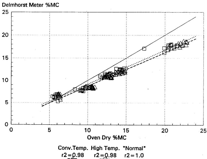
Figure 1. Data and regression lines for red pine tested with a resistance-type meter.
