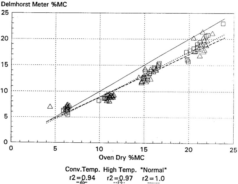
Figure 3. Data and regression lines for eastern hemlock tested with a resistance-type meter.
