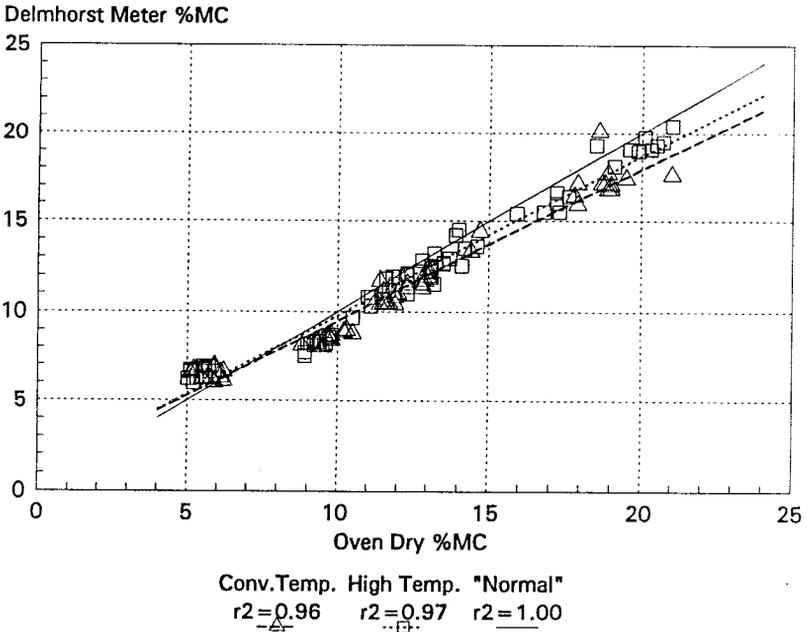
Figure 2. Data and regression lines for eastern white pine tested with a resistance-type meter.
