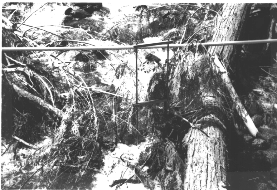
Figure 13. Measuring rod and sampling frame were used to quantify fine and branch-type debris.
