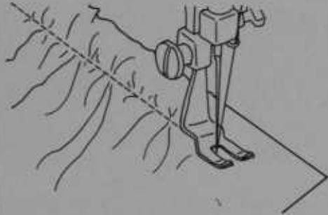
A gathering foot automatically gathers with each machine stitch. The longer the stitch, the closer the gathers will be. Determine the desired closeness and fabric needed by measuring a sample before and after gathering. Refer to your sewing machine manual for directions on operating the gathering foot.
