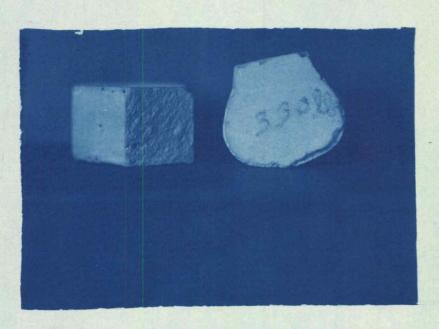
The above briquettetested a tensil strength of 350 lbs.
