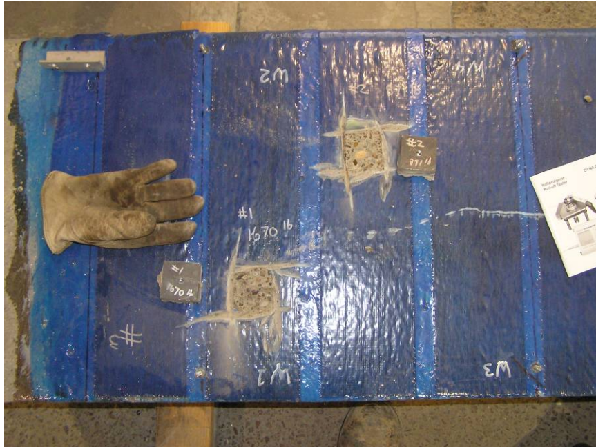
Fig. 4 – Cohesive failure of concrete surface bonded to CFRP caused by direct-tension pull-off tests.
