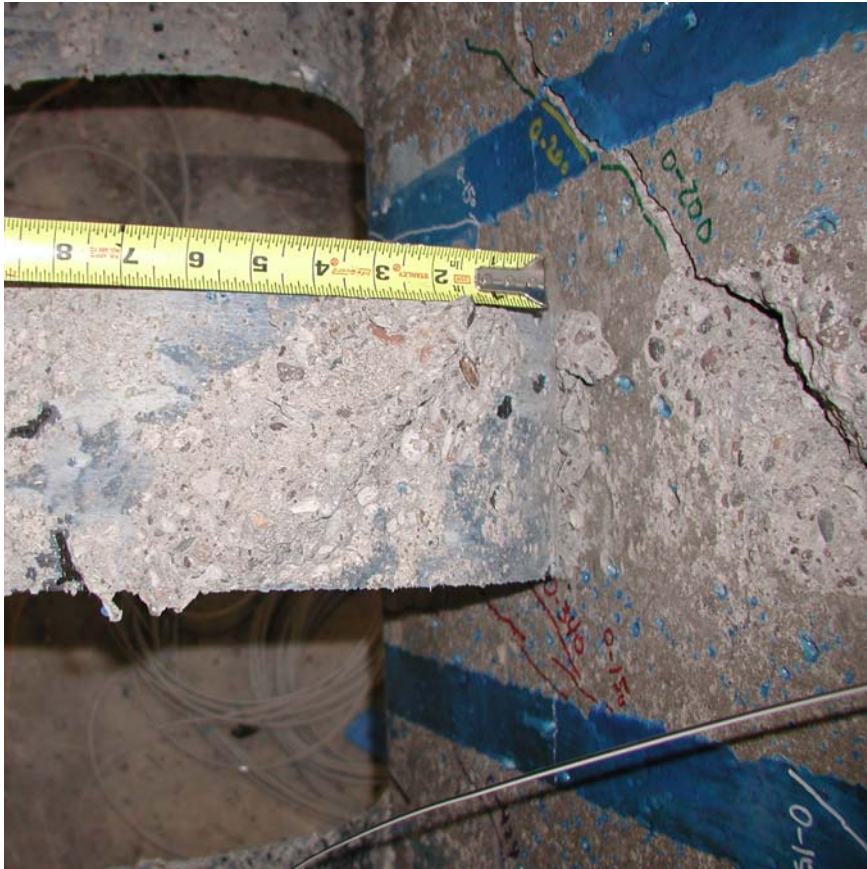
Fig. 30 – Photograph of a debonded CFRP strip that formerly crossed a diagonal crack (post-failure of Specimen FC).
