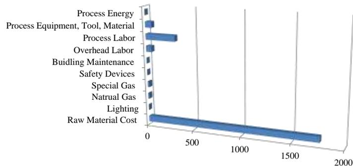
The shopfloor level structure includes some variables the values of which are aggregated by operation level variables. They are process labor ( $C_{\text{Processlabor}}$ ), process equipment tool and material ( $C_{\text{PETM}}$ ), and process energy ( $C_{\text{processenergy}}$ ). Exhibit 6 shows the shopfloor structure cost composition for one unit of product model A.
