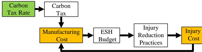
**Figure 5.22. Effect Chain of Carbon Tax Rate on Injury Cost and Manufacturing Cost**
