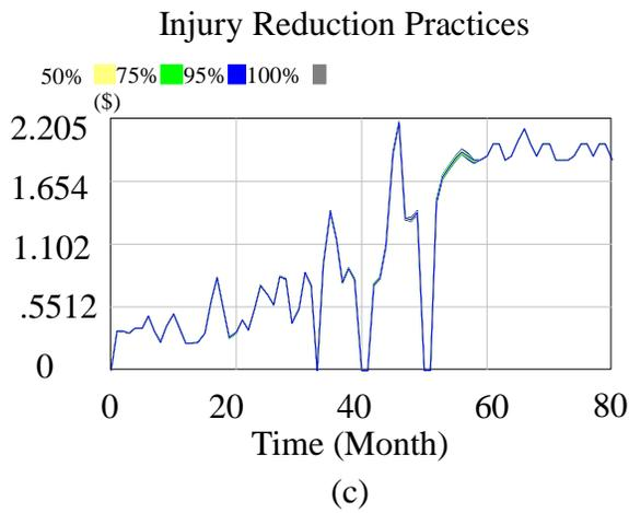
**Figure 5.12. Sensitivity Analysis of Machining Time on (a) Manufacturing Cost, (b) ESH Budget, and (c) Injury Reduction Practices**
