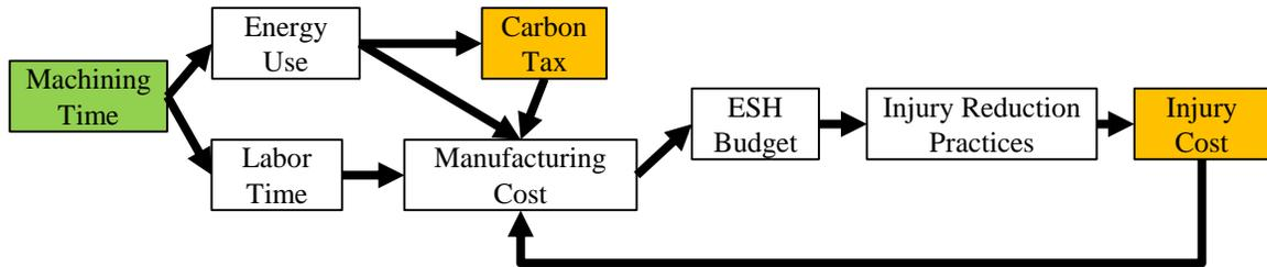
**Figure 5.10. Effect Chain of Machining Time on Carbon Tax and Injury Cost**
