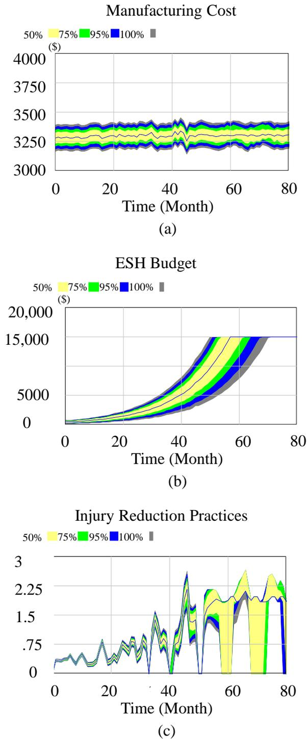
**Figure 5.18. Sensitivity Analysis of Machining Time, Setup Time, and Stainless Steel Use on (a) Manufacturing Cost, (b) ESH Budget, and (c) Injury Reduction Practices**
