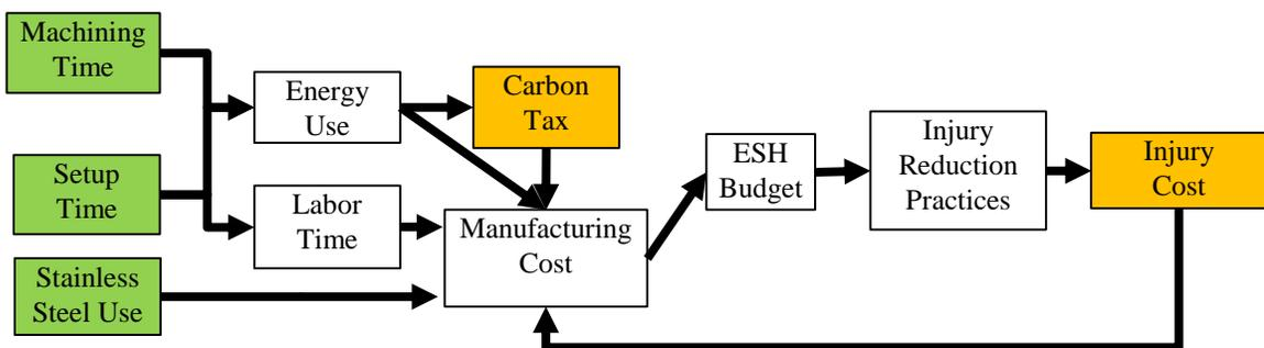
**Figure 5.16. Effect Chain of Simultaneous Change of Machining Time, Setup Time, and Stainless Steel Use on Carbon Tax and Injury Cost**
