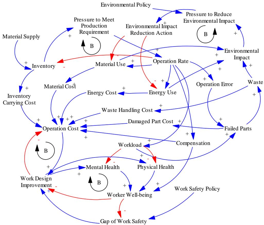
**Figure B.5.** Example Operation Level SD Model.
