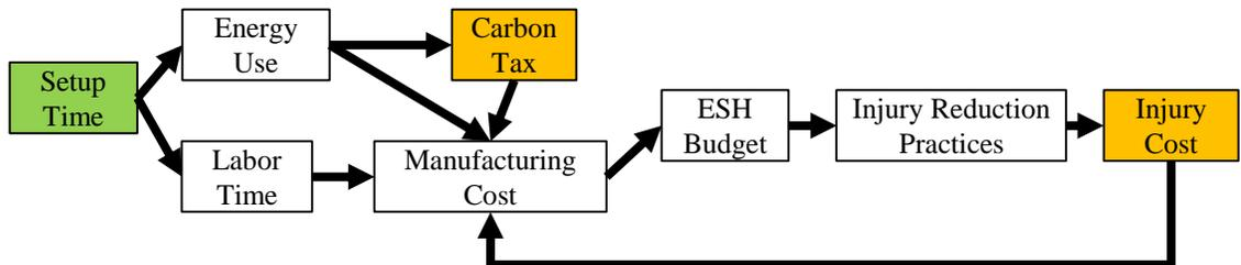
**Figure 5.8. Effect Chain of Setup Time on Carbon Tax and Injury Cost**
