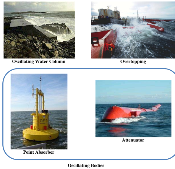
Figure 2.1: Wave Energy Converter Technologies: (from top left) Wavegen Limpet, Wave Dragon, OPT PowerBuoy, and Pelamis [8, 7, 5, 6]
