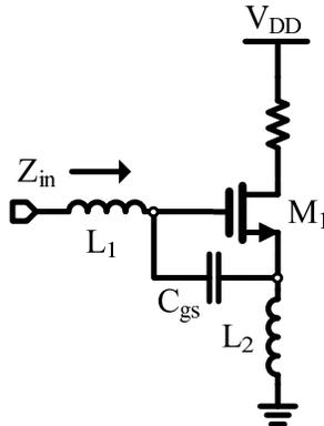
FIGURE 3.4: Inductively degenerated LNA.
