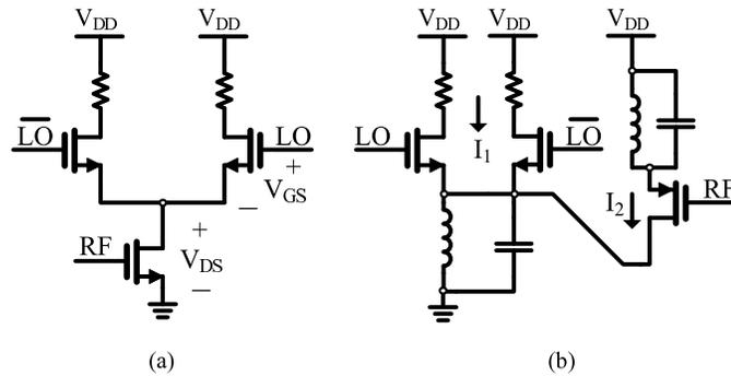
FIGURE 5.1: (a) Traditional single-balanced mixer. (b) Folded single-balanced mixer.
