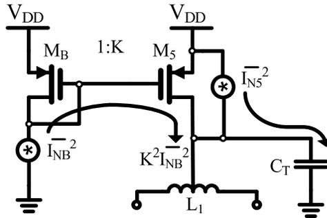
FIGURE 4.3: Effect of tail capacitor and bias noise.
