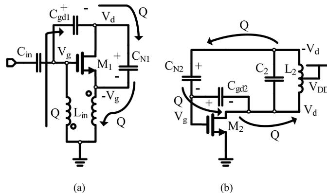
FIGURE 3.8: (a) Stage 1 neutralization. (b) Stage 2 neutralization.
