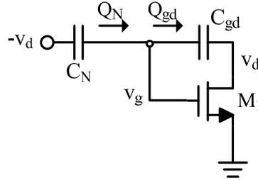
FIGURE 3.7: Basic concept of neutralization.
