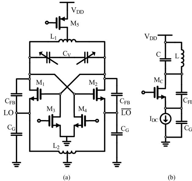
FIGURE 4.1: (a) Circuit schematic of VCO. (b) Traditional Colpitts oscillator.
