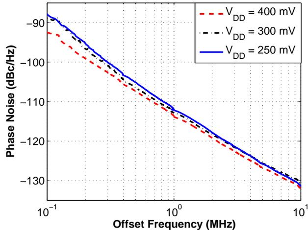
FIGURE 6.5: Measured phase noise of Q channel oscillator.
