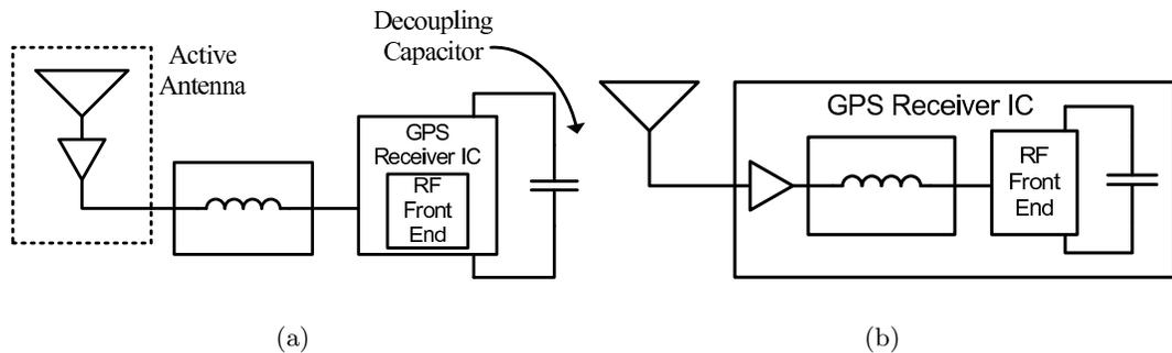
FIGURE 2.1: (a) Typical receiver implementation. (b) Fully integrated receiver.
