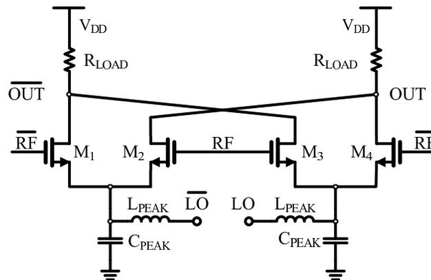
FIGURE 5.2: Double-balanced switched transconductor mixer circuit schematic.
