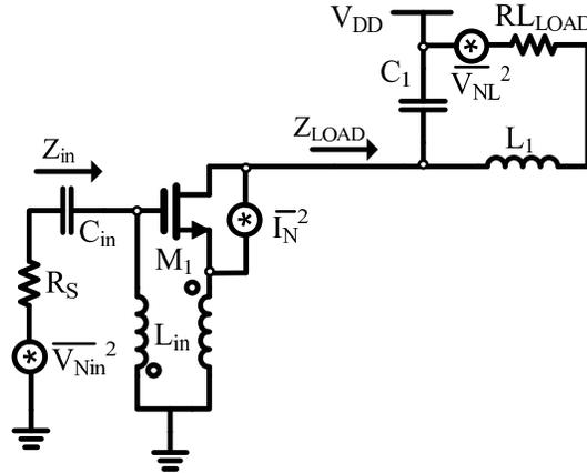
FIGURE 3.10: Schematic of the LNA input stage with noise sources.
