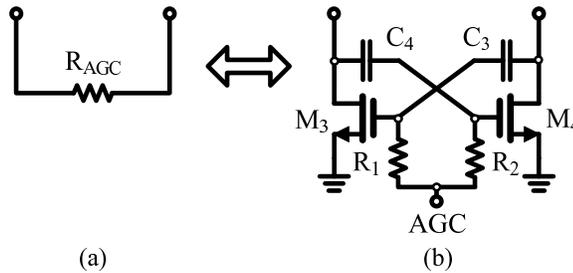
FIGURE 3.12: (a) Simple negative resistor representation of the variable gain circuit. (b) Negative resistance generated by  $M_3$  and  $M_4$  for variable gain.
