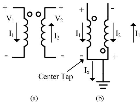
FIGURE 3.2: (a) Voltage and current in a transformer. (b) Voltage and current in a center tapped inductor.
