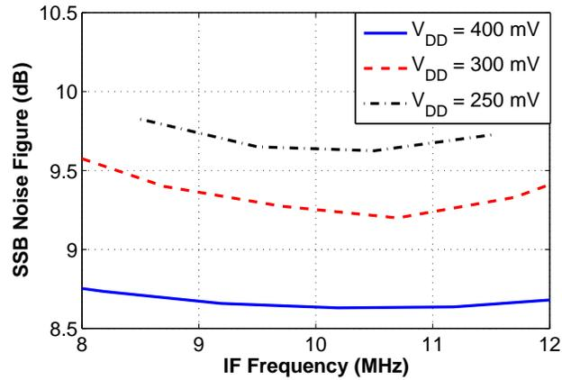
FIGURE 6.3: Measured noise figure.
