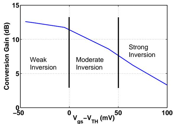
FIGURE 5.3: Simulated conversion gain vs. transconductor operating region.
