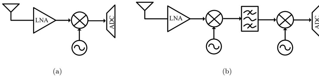
FIGURE 2.2: (a) Direct conversion architecture. (b) Superheterodyne architecture.
