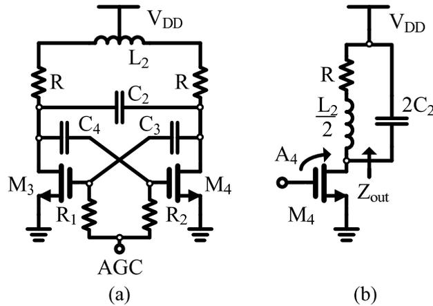
FIGURE 3.11: (a) Variable gain circuit in second stage of LNA. (b) AC half circuit of variable gain circuit.
