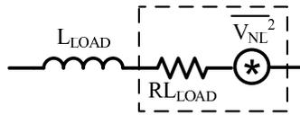
FIGURE 3.9: Inductor noise model.
