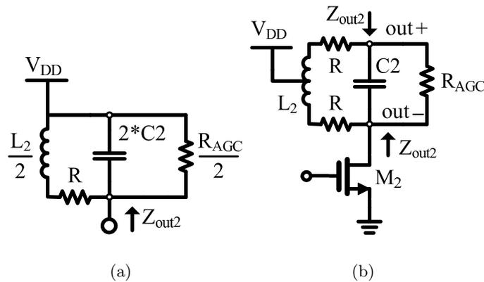
FIGURE 3.13: (a) Output impedance to common mode. (b) Simplified schematic to analyze gain of stage 2.
