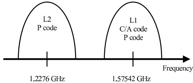
FIGURE B.1: Typically used GPS bands.
