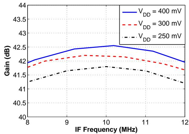
FIGURE 6.4: Measured gain.
