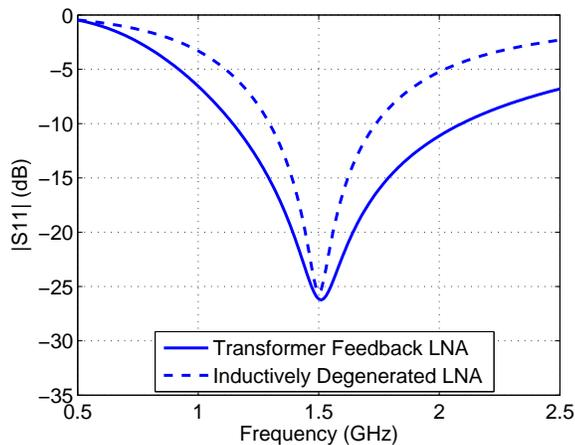
FIGURE 3.6:  $|S_{11}|$  for inductive degeneration and transformer feedback input matching.
