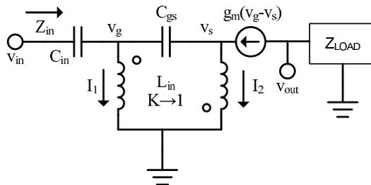
FIGURE 3.3: AC model of the LNA input.
