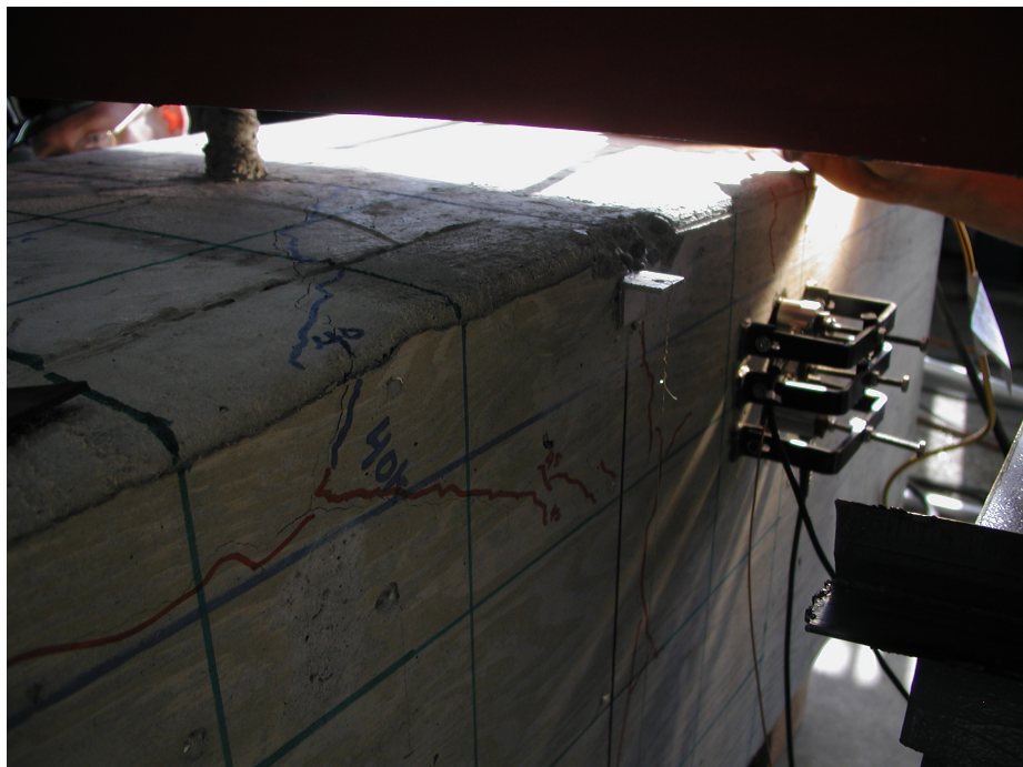
Fig. R28 Picture of Specimen 1M08.21 prior to failure, with cracking observed.
