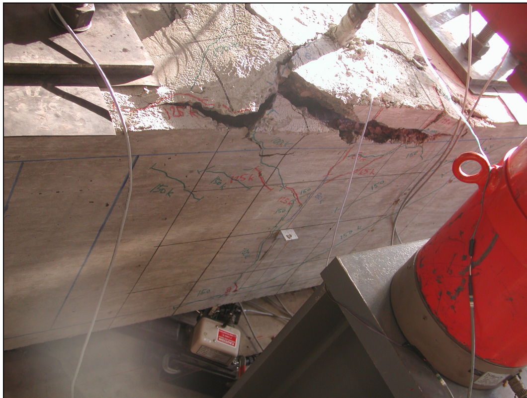
Fig. R33 - Specimen 2L0.21 at failure.
