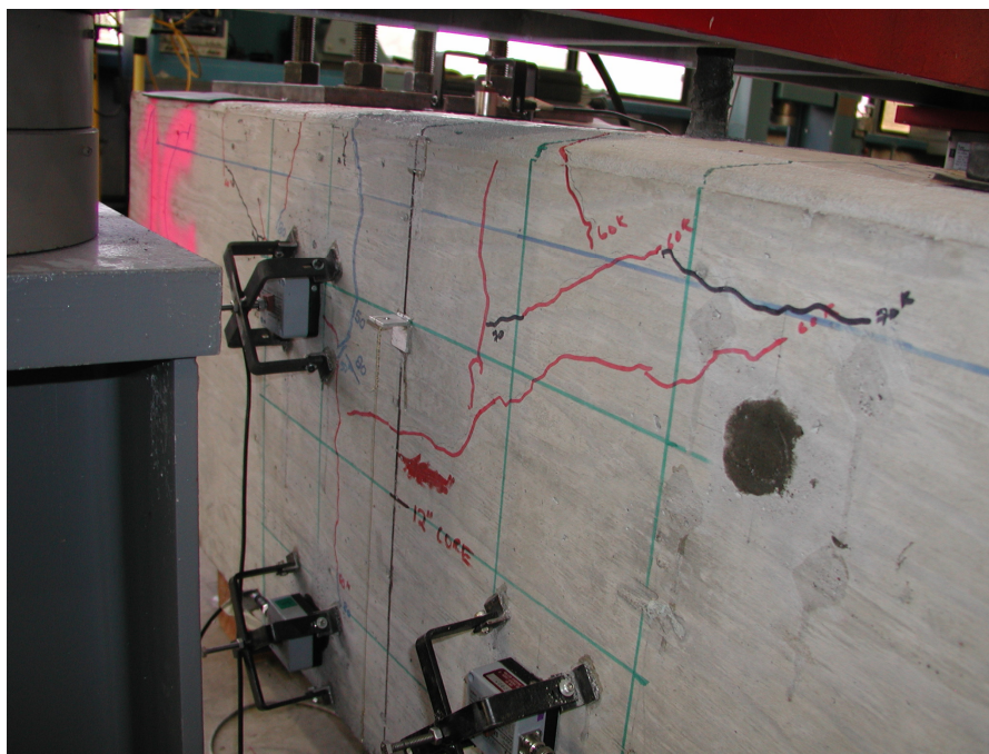
Fig. R29 - Picture of Specimen 1M12.21 near failure, with cracking observed.
