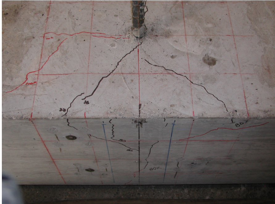
Fig. R30 - Picture of Specimen 1M0.21 at failure, with cracking observed.
