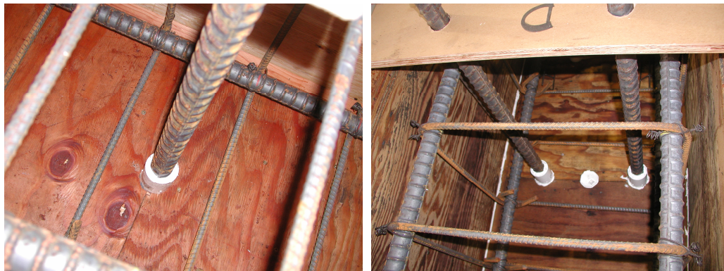
Fig. R7-Typical PVC debonding pipe placed in specimens prior to casting.
