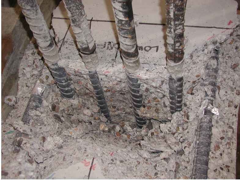
Fig. R19 - Visible concrete wedge penetration, concrete still in contact with reinforcing after failure.
