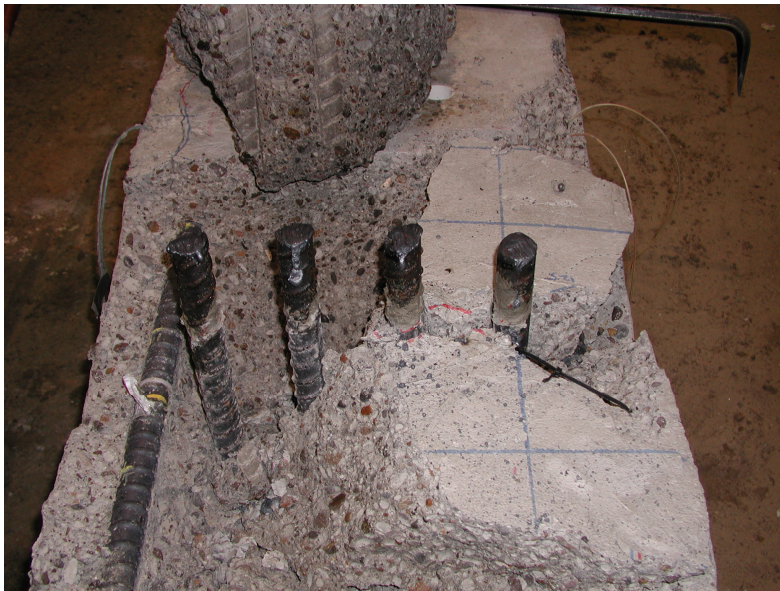
Fig. R20 - Failure of Specimen with concrete wedge, bar imprint visible.
