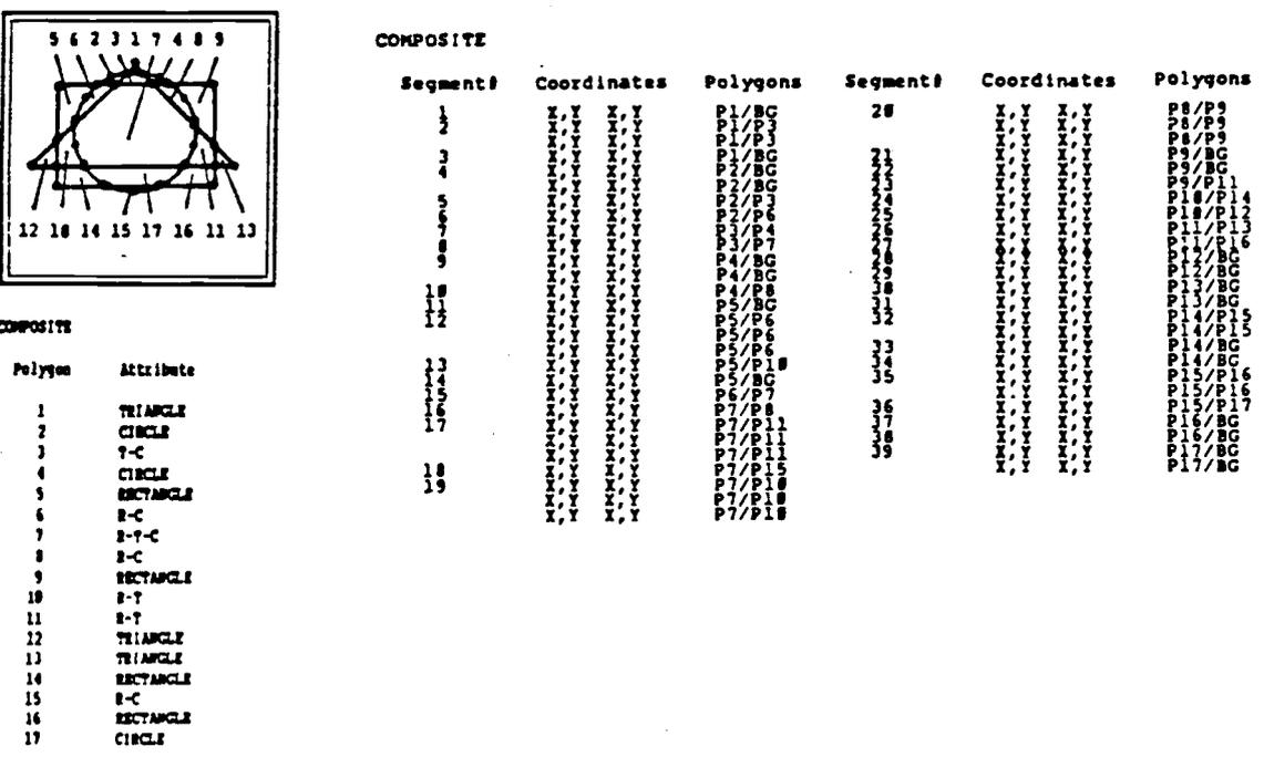
Figure 1. An example of vector data. The coordinate data is at the right of each figure. The initial storage needs are small and the data structure relatively simple. When the three figures are overlaid the increase in complexity and storage is quite large (Berry, 1989).
