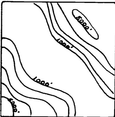
The first is a topographic map constructed to show the surface of the earth as a set of lines connecting locations of equal elevation.
