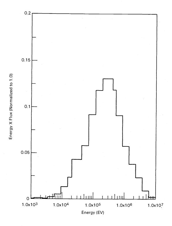
FIGURE 3. ACT6X9 Oxide Spectrum in an Infinite EBR-II Configuration
