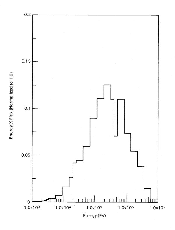
FIGURE E8. ACT6X9 Carbide Spectrum in an Infinite GCFR Configuration
