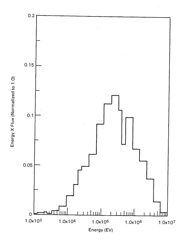
FIGURE 4. ACT6X9 Carbide Spectrum in an Infinite EBR-II Configuration
