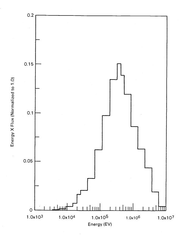
FIGURE E6. ACT6X9 50 wt % Molybdenum Spectrum in an Infinite GCFR Configuration
