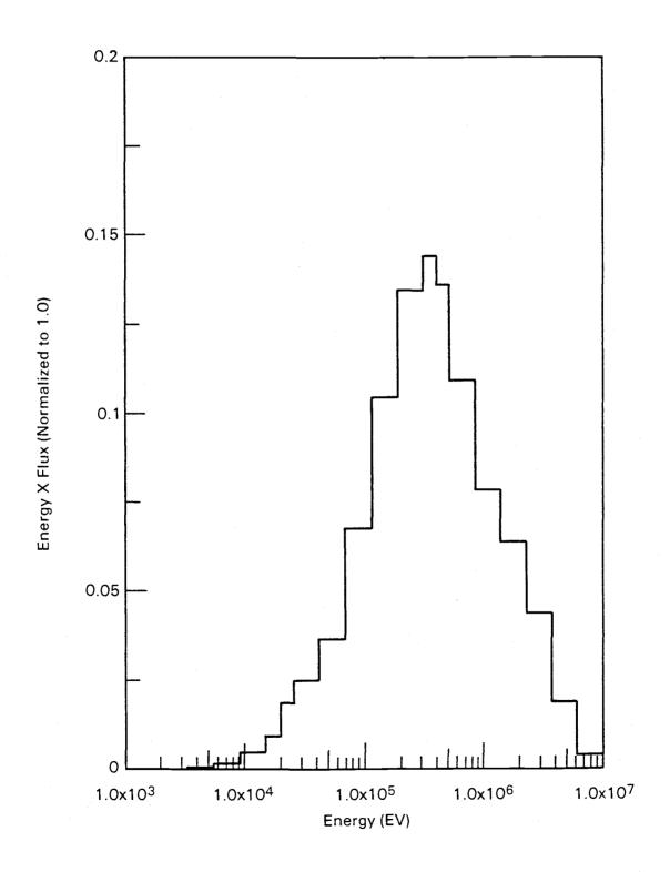
FIGURE E2. ACT6X9 50 wt % Molybdenum Spectrum in an Infinite LMFBR Configuration
