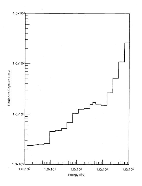
FIGURE B3. Am-243 Fission-to-Capture Ratio as a Function of Energy
