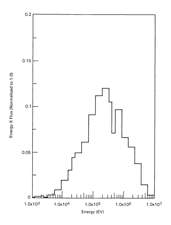
FIGURE E4. ACT6X9 Carbide Spectrum in an Infinite LMFBR Configuration
