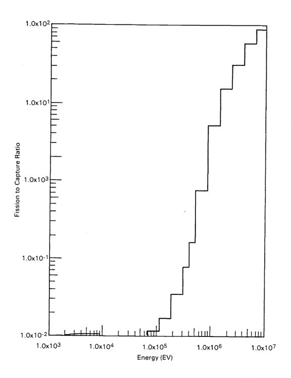
FIGURE B2. Am-242m Fission-to-Capture Ratio as a Function of Energy
