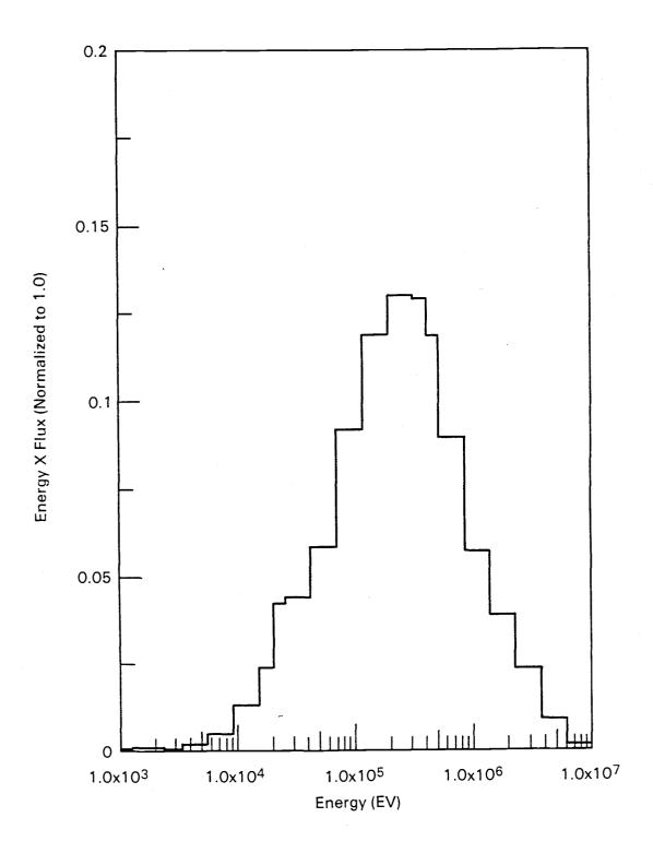
FIGURE E3. ACT6X9  $0\times$ ide Spectrum in an Infinite LMFBR Configuration
