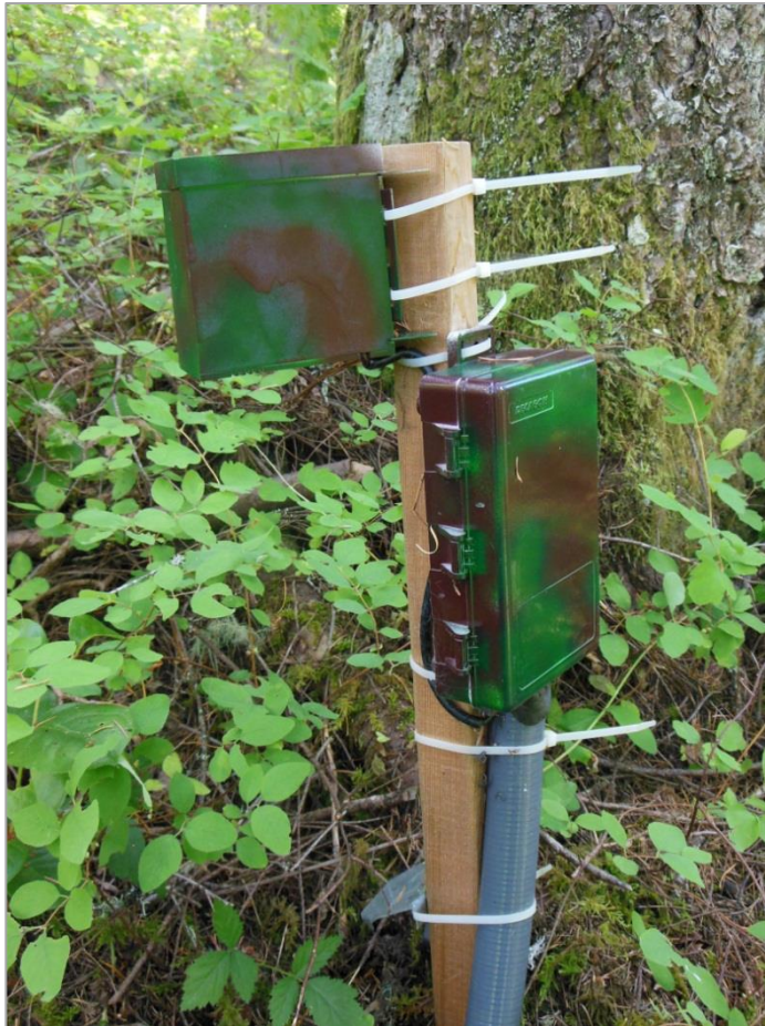
Figure 3-2: Mini-meteorological station established for monitoring soil volumetric water content ( \text{m}^3/\text{m}^3 ) at two-hour intervals.
