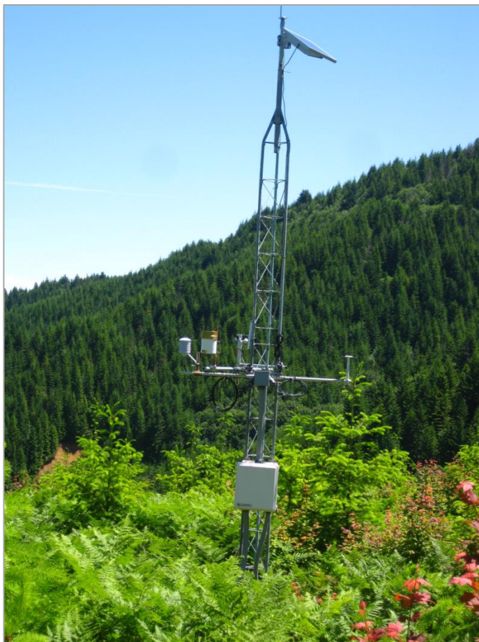
Figure 4-4: Mega-meteorological station established at Panther Creek for collecting detailed climatic data.
