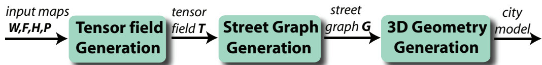
Figure 2.6: The modeling pipeline. Stage 1 is the tensor field design stage, roads are extracted in stage 2, and stage 3 is a geometry creation stage.
