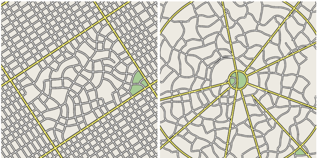
Figure 4.5: Noise produces curved minor roads over major roads. Left: Over a regular major road grid. Right: Over a radial major road grid.
