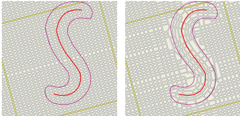
Figure 4.2: Example of the brush stroke interface. The image on left shows the network before the brush stroke was applied and right shows the effects of the brush stroke.
