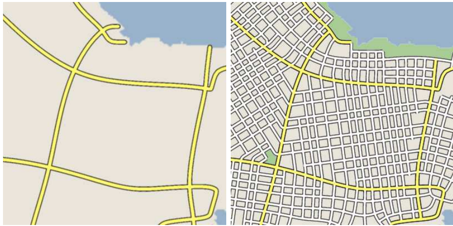
Figure 5.3: The major roads (left) are used to segment the editing domain for the minor roads (right).
