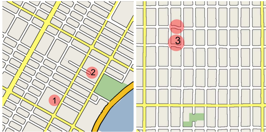
Figure 6.2: Sometimes cells are merged (1) or partially split by dead ends (2). Regular grids sometimes suffer slight shifts (3).
