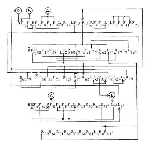
Figure 3. The operator program of the QL and AL mode of NAC. For complete description, refer to the quintuple list in Figure 5.
