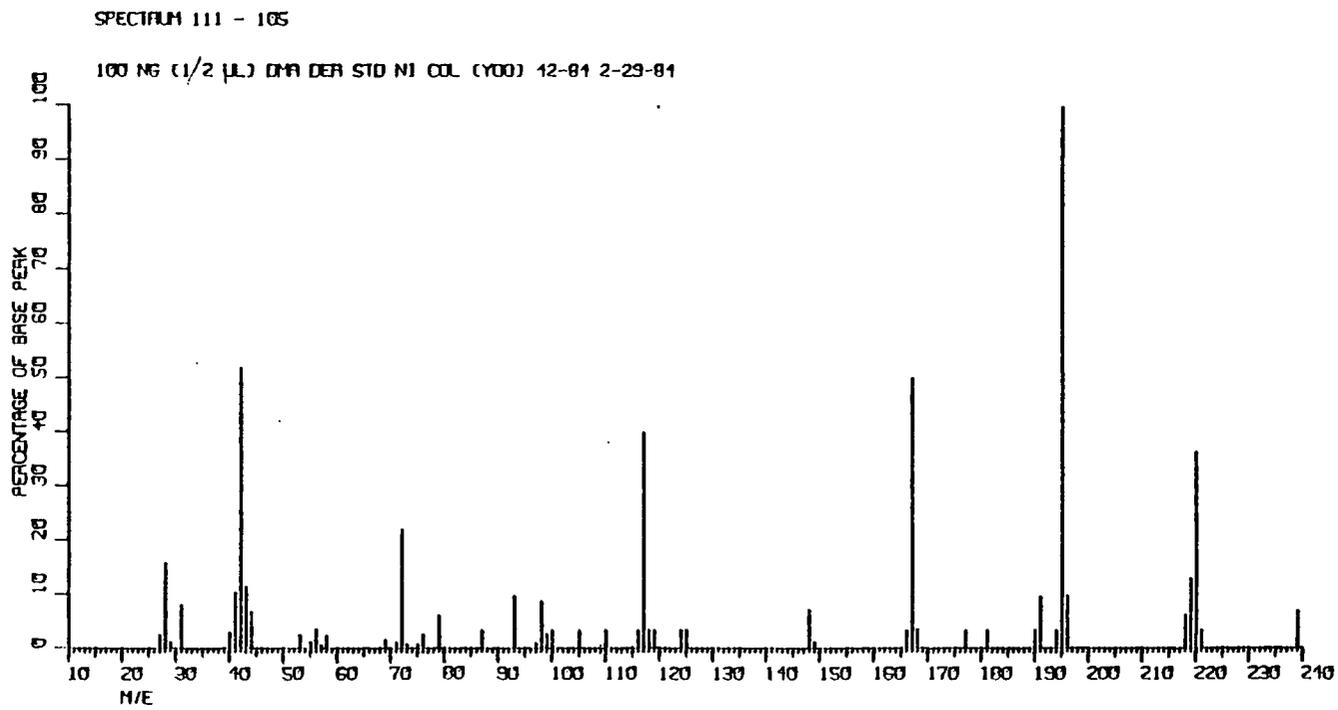
Figure 10. Mass spectrum of dimethylamine derivative
