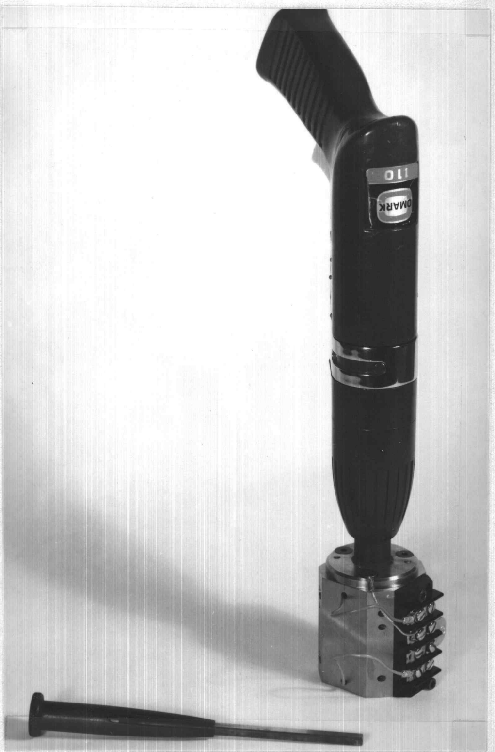
Figure 3. Powder actuated tool, transducer, and power plug.
