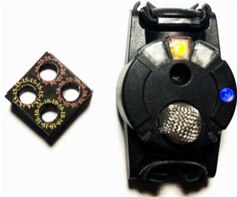
Shockwave Exposure Indicator, latest version, June 2020 (*left*) and Blast Gauge (*right*).
