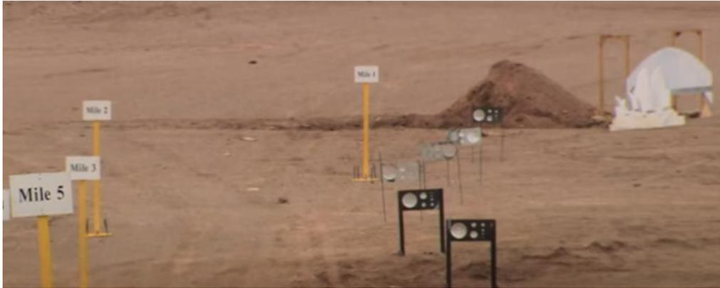
Bikini Gauges used to estimate blast force from scaled recreation of a meteor impact with TNT, illustrating scalability of the gauge's application. [110]
