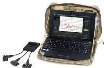
(Left) Blast Gauge Field Testing-Afghanistan, 2014. [112] (Right) Blast Gauge System. [113]
