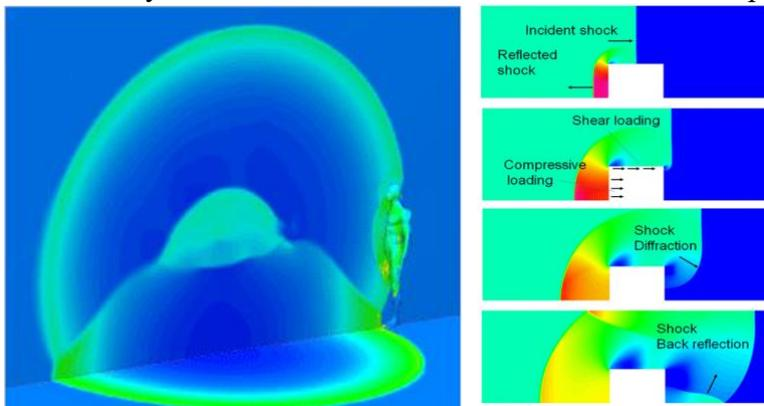
(Left) Blast wave impulse from M67 fragmentary grenade. [114]
