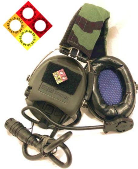
Shockwave Exposure Indicator prototype affixed to hearing protection.
