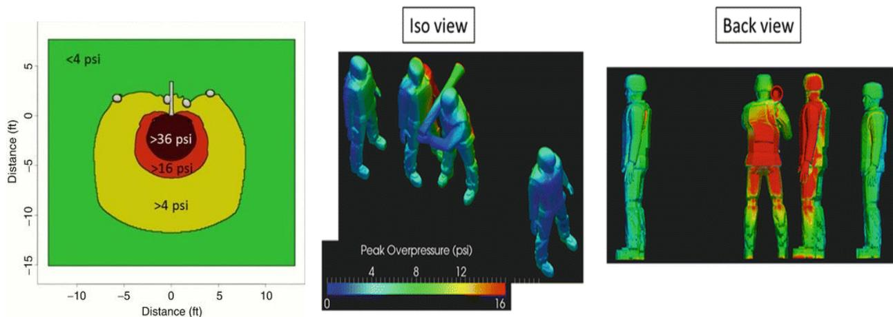
Diagram displaying blast overpressure impulse levels from an M-48 Carl Gustav Recoilless Rifle.[87]
