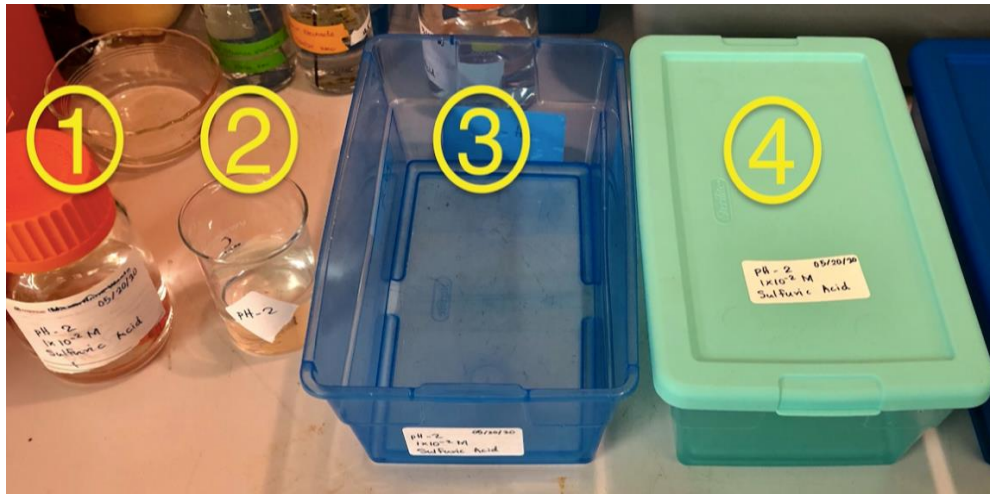
Figure-A1: 1). Close glass, 2). Open glass, 3). Open plastic, and 4). Close plastic containers of sulfuric acid solution without any samples.
