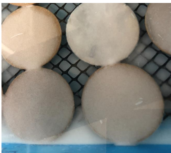
Figure-2.10: The precipitation in white color around the specimens in pH2 sulfuric acid solution after 14 days.
