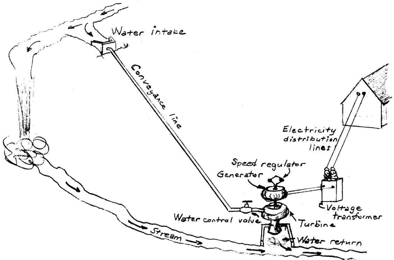
Figure 1. Components of a typical backyard hydropower system.
