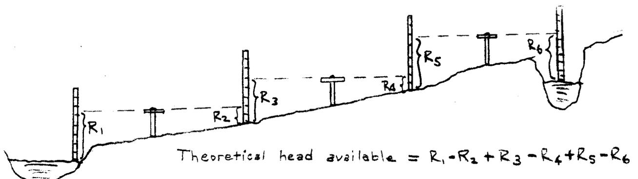
the rising ground. The level and level rod are moved alternately. Two people are needed. Still better estimates can be obtained by use of a surveyor's level (or transit) and leveling rod.
