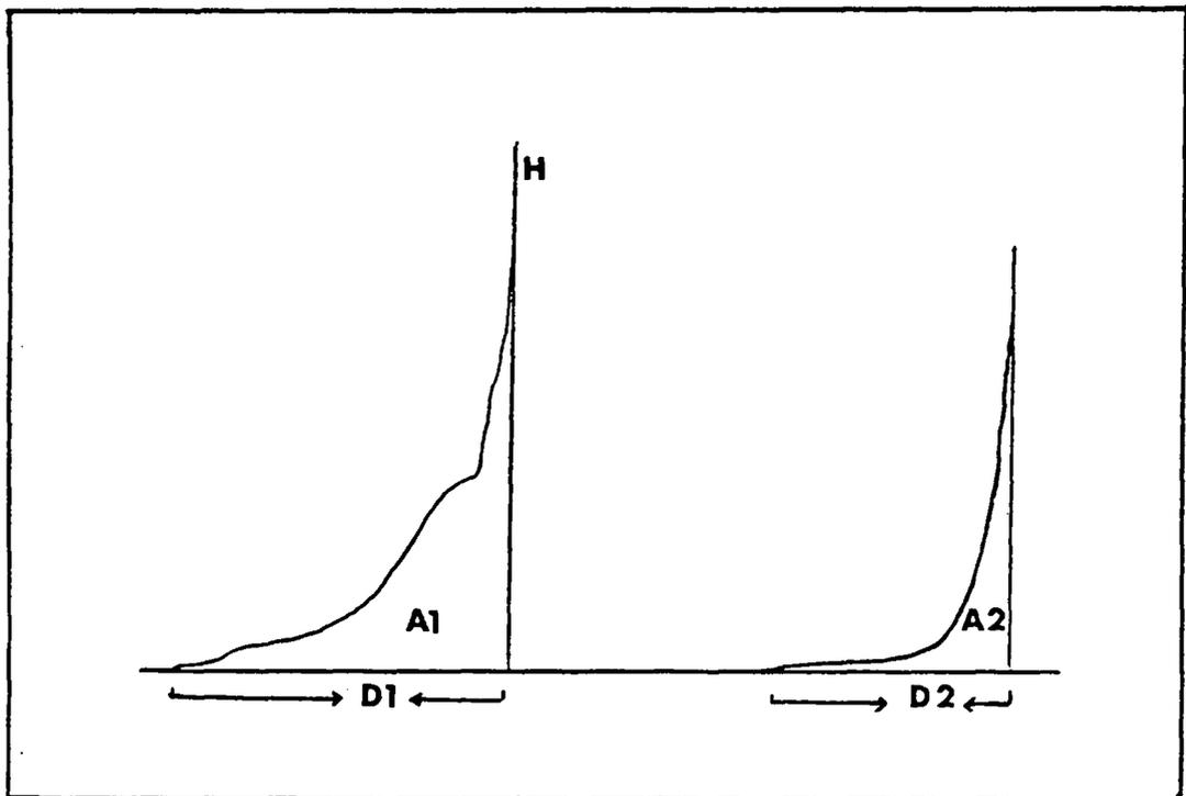
Figure 3. Instrumental Texture Profile Analysis (ITPA) from a Pacific whiting cooked gel. Double bite test. Hardness (H) in pounds; cohesiveness ( $A2/A1$ ); elasticity ( $D2/D1$ ) x (100).
