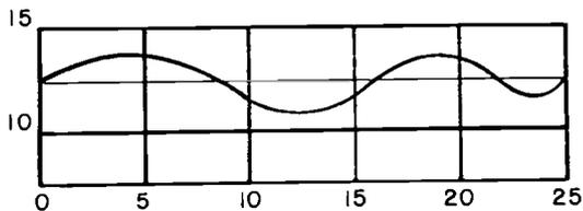
We now lay a grade which we feel is balanced so that the excavation will make the embankment:
