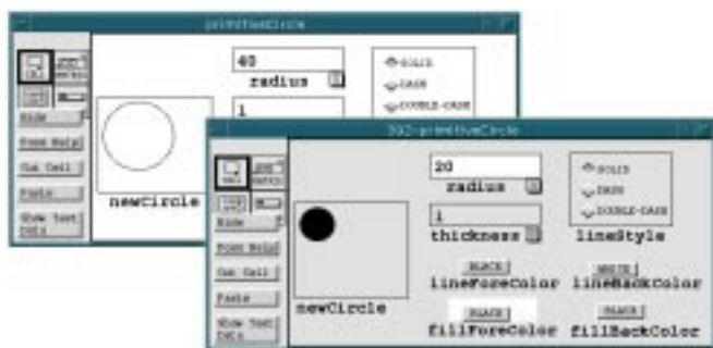
Figure 1: The white primitiveCircle form is a built-in form that defines a prototypical instance of type primitiveCircle. The gray 392-primitiveCircle form is a copy that has been modified to describe a different instance. The circle in cell newCircle is defined by the other cells, which specify its attributes. To refer to the circle elsewhere in the program, a formula can reference 392-primitiveCircle:newCircle. The programmer cannot view the formula (primitive implementation) of newCircle, but can view and specify the other cells' formulas by clicking on their formula tabs (■). Radio buttons and popup menus (e.g., lineForeColor) provide a way to reliably enter constant formulas when only a limited set of constants are valid.
