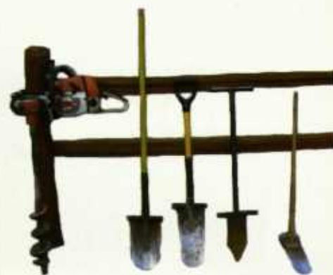
Figure 6.2. Planting tools include the power auger (at left), various types of shovels, and the hoedad (at right).
