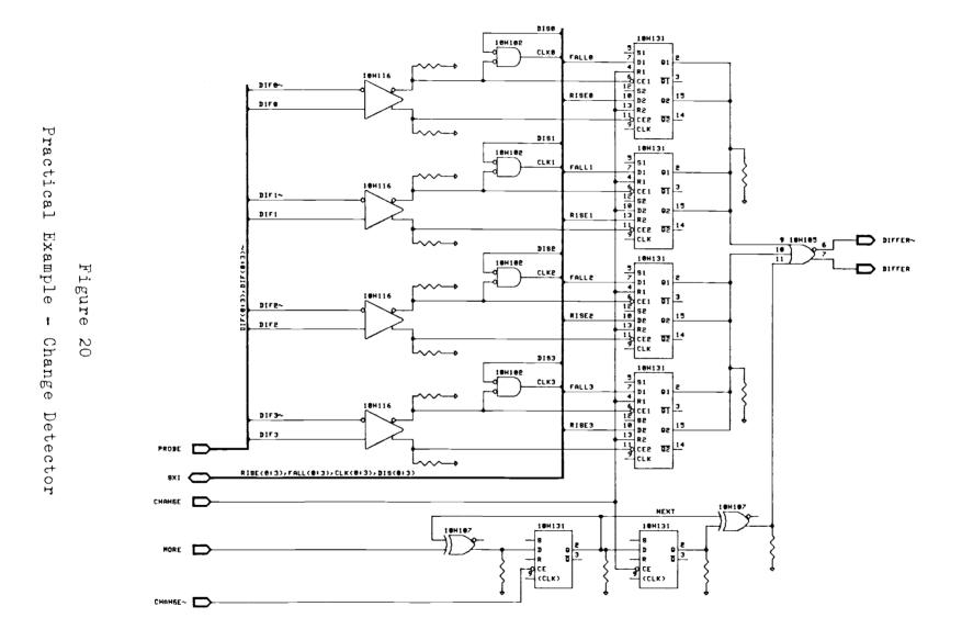
accommodated and, by enabling both flip-flops, a levelsensitive input can be accommodated. The choice is made by programming the signals RISE(0:3) and FALL(0:3). A high on the appropriate signal enables a clock pulse while a low inhibits a clock pulse on that edge.
