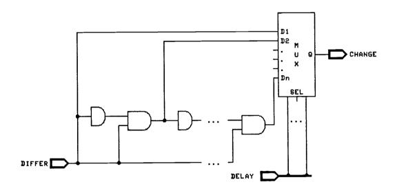
Figure 4 Programmable Asymmetrical Delay
