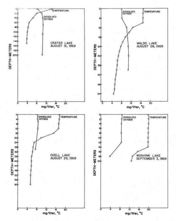
Figure 3. Temperature and dissolved oxygen profiles compared among four oligotrophic lakes in Oregon. Thermal-D. O. profiles for Odell Lake are shown in the lower left-hand panel. Thermal profiles were determined with a Whitney portable thermometer (model TC-5A) which has a meter scale calibrated in 0.1°C units.
