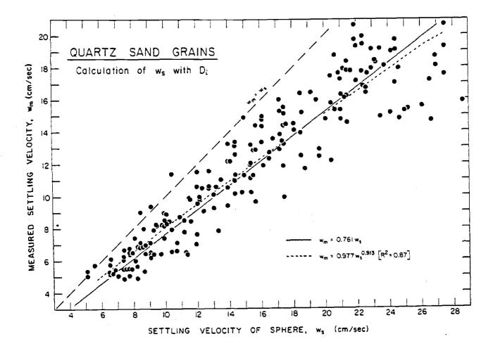
Figure 3: The measured settling velocity,  $w_{\rm m}$ , versus the settling rate of a sphere,  $w_{\rm s}$ , calculated with equation (1) using  $r=D_{\rm i}/2$ .
