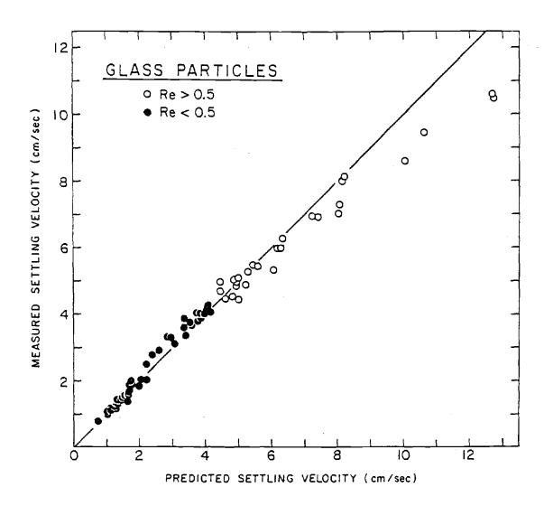
Figure 3: The measured settling velocity  $w_S$  prediction by equation (4). The data in the Stokes region (Re < 0.5) show good agreement (R<sup>2</sup> = 0.986) but the data for Re > 0.5 show a progressive departure.
