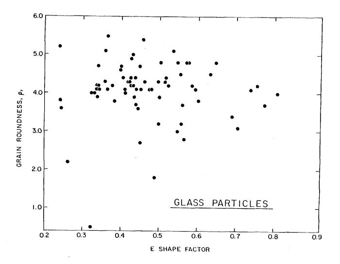
a source from broken beer, wine and pop bottles (in spite of Oregon's bottle bill). The densities of several popular beverage bottles were determined by weighing them and obtaining their volumes by immersion in water contained in a graduated cylinder. The average density was found to be  $2.41 \text{ g/cm}^3$  (total range  $2.39-2.44 \text{ g/cm}^3$ ). This average value is used throughout the analyses for the particle densities.
