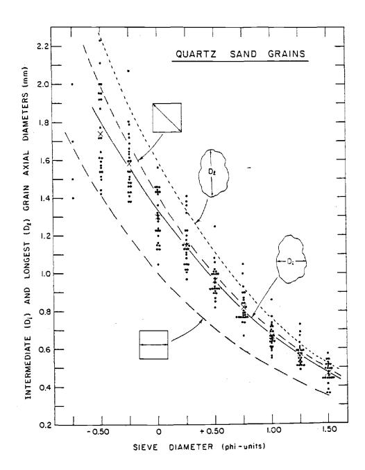
Figure 1: The intermediate diameter  $D_i$  versus the sieve diameter for the 229 quartz sand grains. The two long dashed curves are the diagonal and transverse openings of the sieve screens as shown. Also given as the short-dashed curve is the fit to the means of the longest axial diameters,  $D_1$ .
