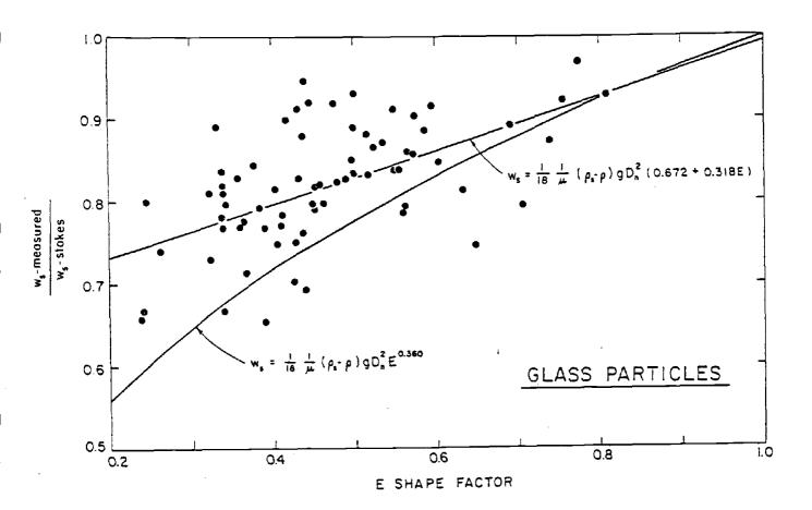
Figure 2: Comparison of the settling velocity to the E shape factor.
