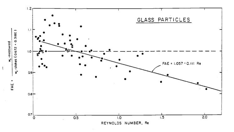
Figure 5: Dependence of the settling velocity on the Reynolds number, showing an approximate linear departure from equation (4) for Re > 0.5. The straight-line fit shown yields equations (5) and (6).
