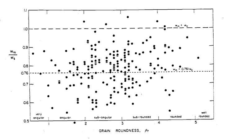
Figure 5: Comparison of the measured settling velocity divided by the calculated settling rate of an "equivalent sphere" with the grain roundness, demonstrating no dependence.
