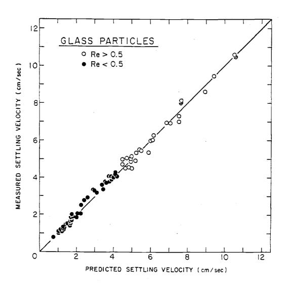
Figure 6: The measured settling velocity versus  $w_S$  predicted by equation (6). A comparison with Fig. 3 shows that equations (4) and (6) are equally good for Re < 0.5, but equation (6) gives much better results for Re > 0.5. The over-all fit is  $R^2$ = 0.99.
