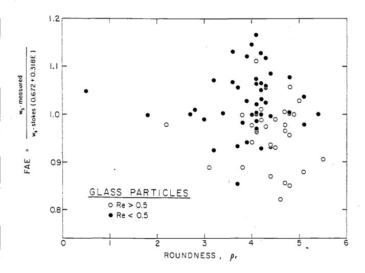
Figure 4: The measured settling velocities, normalized to remove the effects of grain shape, compared to the measured grain roundness, demonstrating the lack of any dependence.
