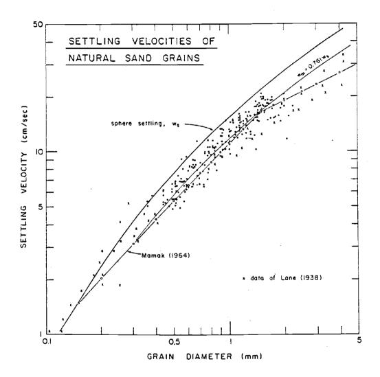
Figure 2: The measured settling velocity versus the grain diameter, taken as  $D_i$  for the data of this study. The upper heavy curve is for the settling of spheres.
