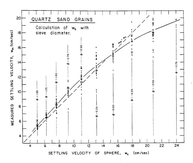
Figure 4: A comparison of the measured settling velocity,  $\mathbf{w}_{\rm m}$  , with the settling rate of a sphere calculated with equation (1) using the sieve diameter.
