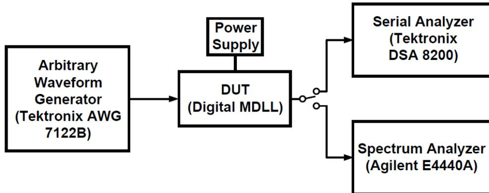
Fig 4.2 Digital MDLL Test Setup
