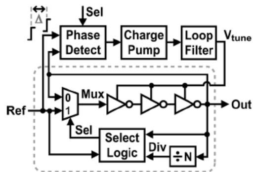
Fig 1.2.3 Analog MDLL Block Diagram [8]
