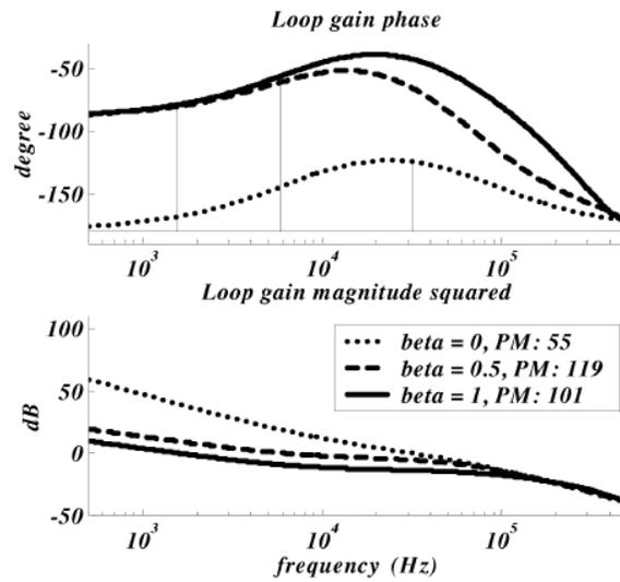
Fig 2.1.6 Effect of Beta on Loop Gain [6]
