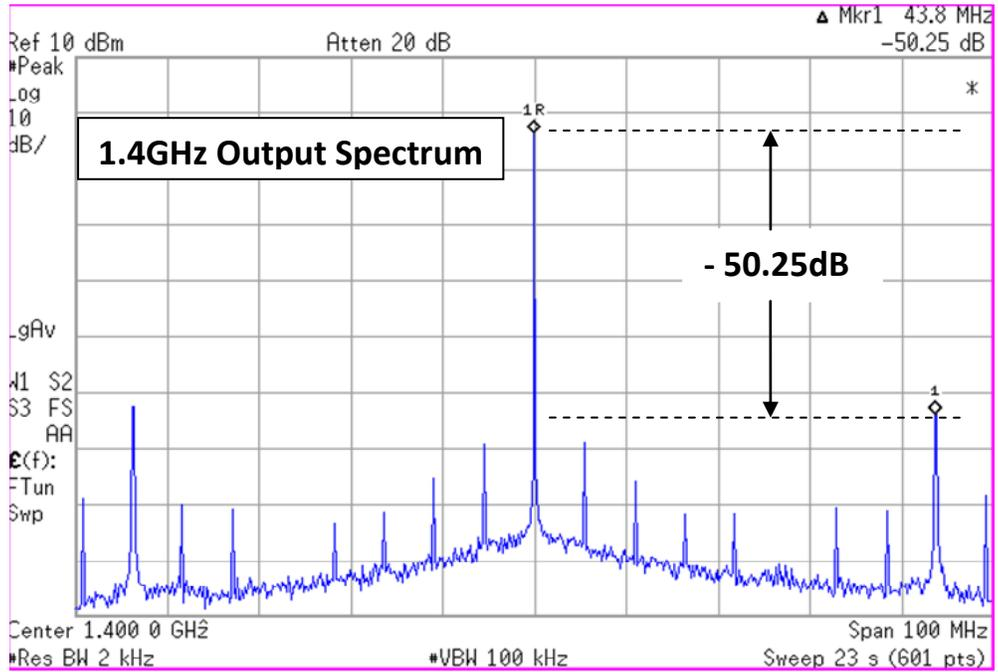
Fig 4.6 Measured Reference Spur at 1.4GHz Output
