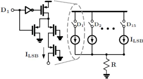
Fig 3.2.4 DAC Current Element
