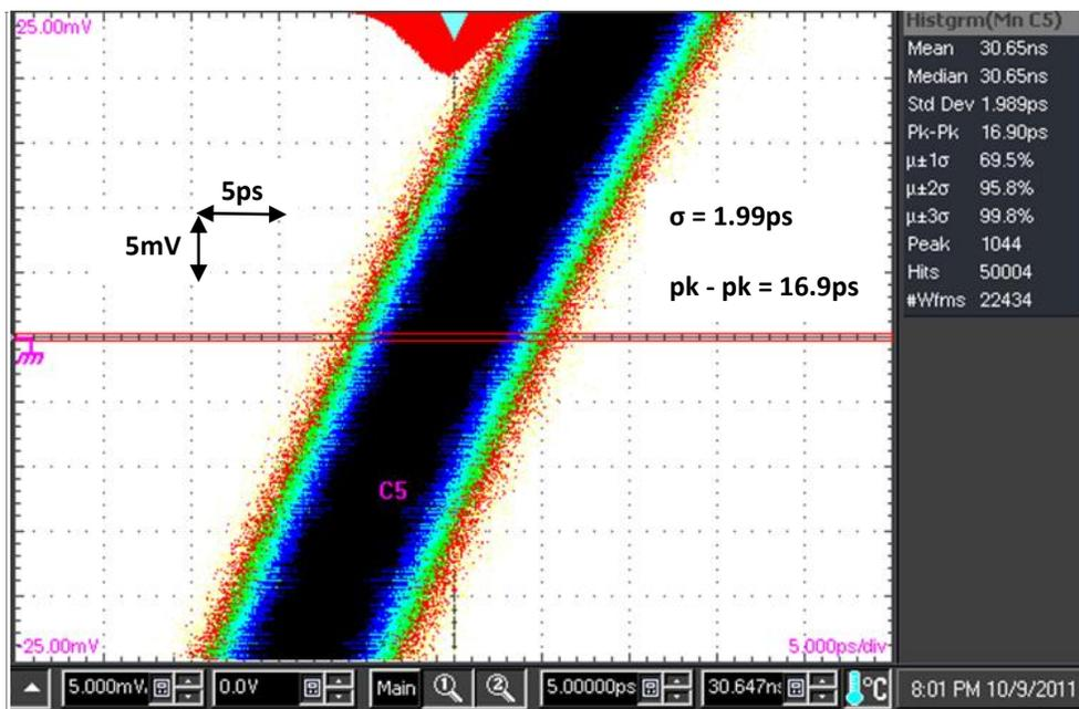
Fig 4.3 Jitter Histogram at 1.4GHz (50K Hits)
