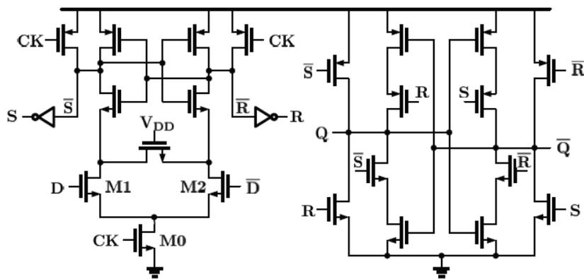
Fig. 3.1.1 Sense Amplifier Flip-Flop Schematic
