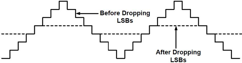
Fig 3.2.1 Limit Cycle in MDLL
