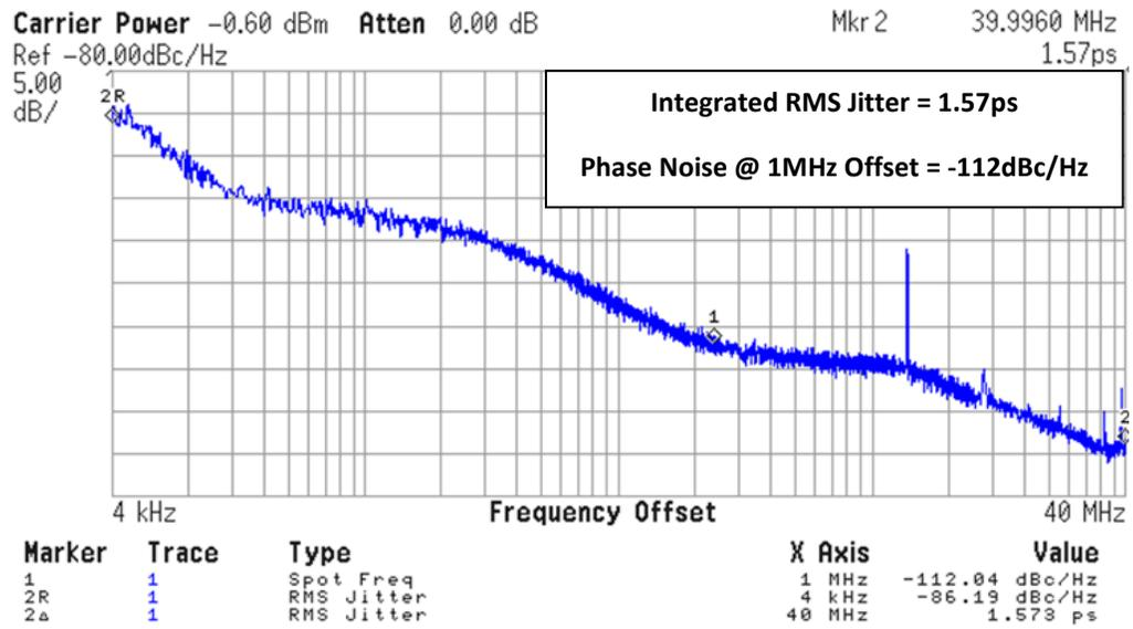
Fig 4.7 Measured Phase Noise at 1.4GHz Output
