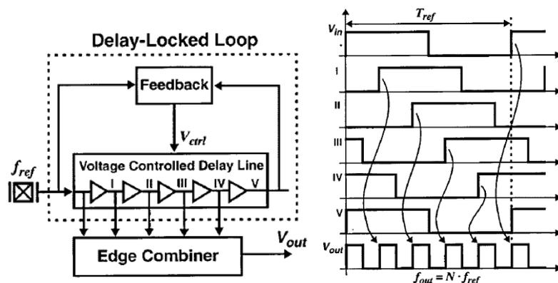
Fig 1.2.1 DLL-based frequency multiplier block diagram and concept [5]
