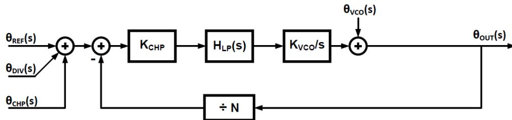
Fig 2.1.1 Phase Noise Model of a Conventional Integer-N PLL [6]
