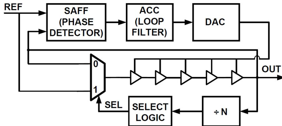
Fig 3.1 Proposed MDLL Architecture
