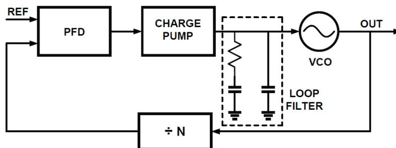
Figure 1.1.2 CPPLL Block Diagram
