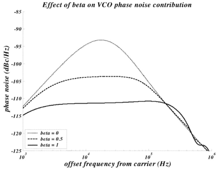
Fig 2.1.5 Phase Noise Filtering by RPLL [6]
