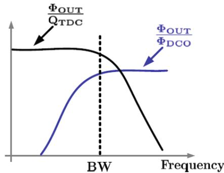
Fig 2.2.1 Noise Bandwidth Tradeoff in Digital PLL
