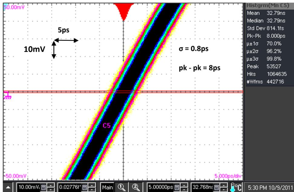
Fig 4.5 Reference Clock Jitter Histogram at 43.75MHz (1M Hits)
