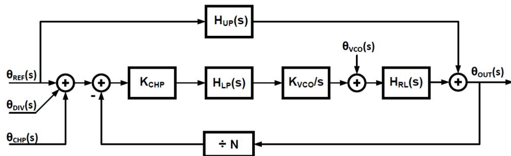
Fig 2.1.2 Phase Noise Model of a Realigned PLL [6]
