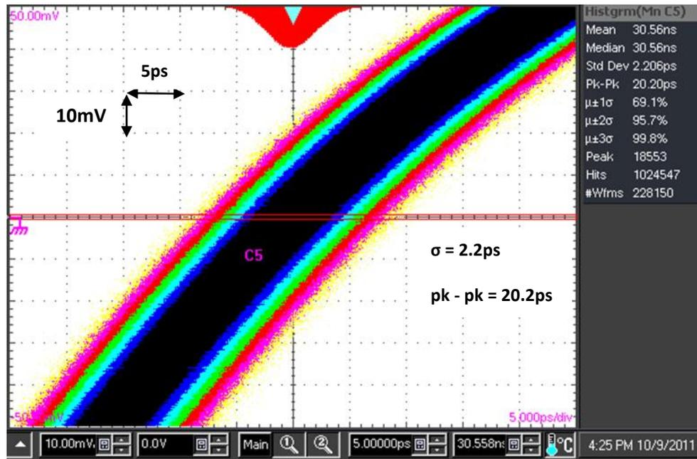
Fig 4.4 Jitter Histogram at 1.4GHz (1M Hits)
