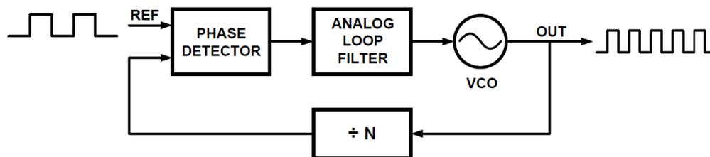
Figure 1.1.1 PLL Block Diagram
