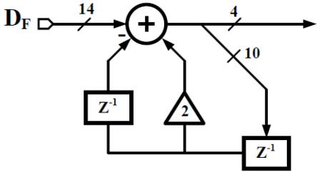
Fig 3.2.3 Delta Sigma Modulator
