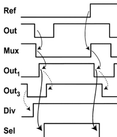
Fig 3.4.2 SELECT Logic Timing Diagram
