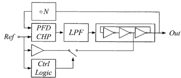
Fig 1.2.2 Realigned PLL Block Diagram [6]
