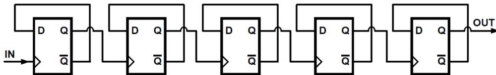
Fig 3.5.1 Divider Using TSPC Flip-Flop
