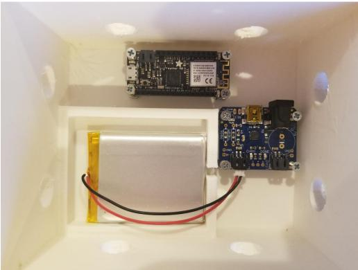
Figure 4.7: 3D Printed Enclosure with PCB
