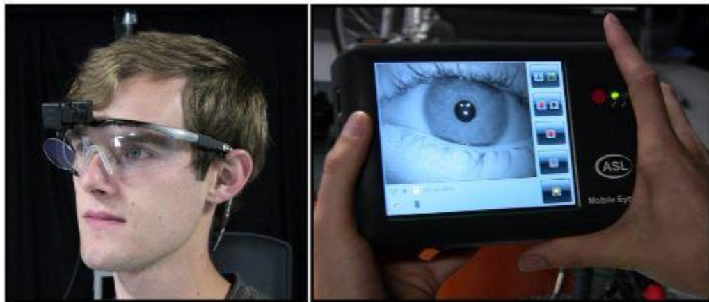
Figure 9: OSU Researcher Demonstrating the Mobile Eye XG Glasses and Mobile Recording Unit
