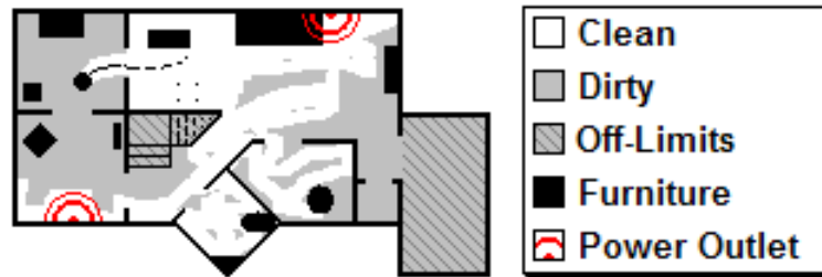
Figure 3.3: Example Environment for Position-Based Representation - a static world where rewards are only dependent on the robot's location is ideal for a representation that is defined by its global coordinates.
