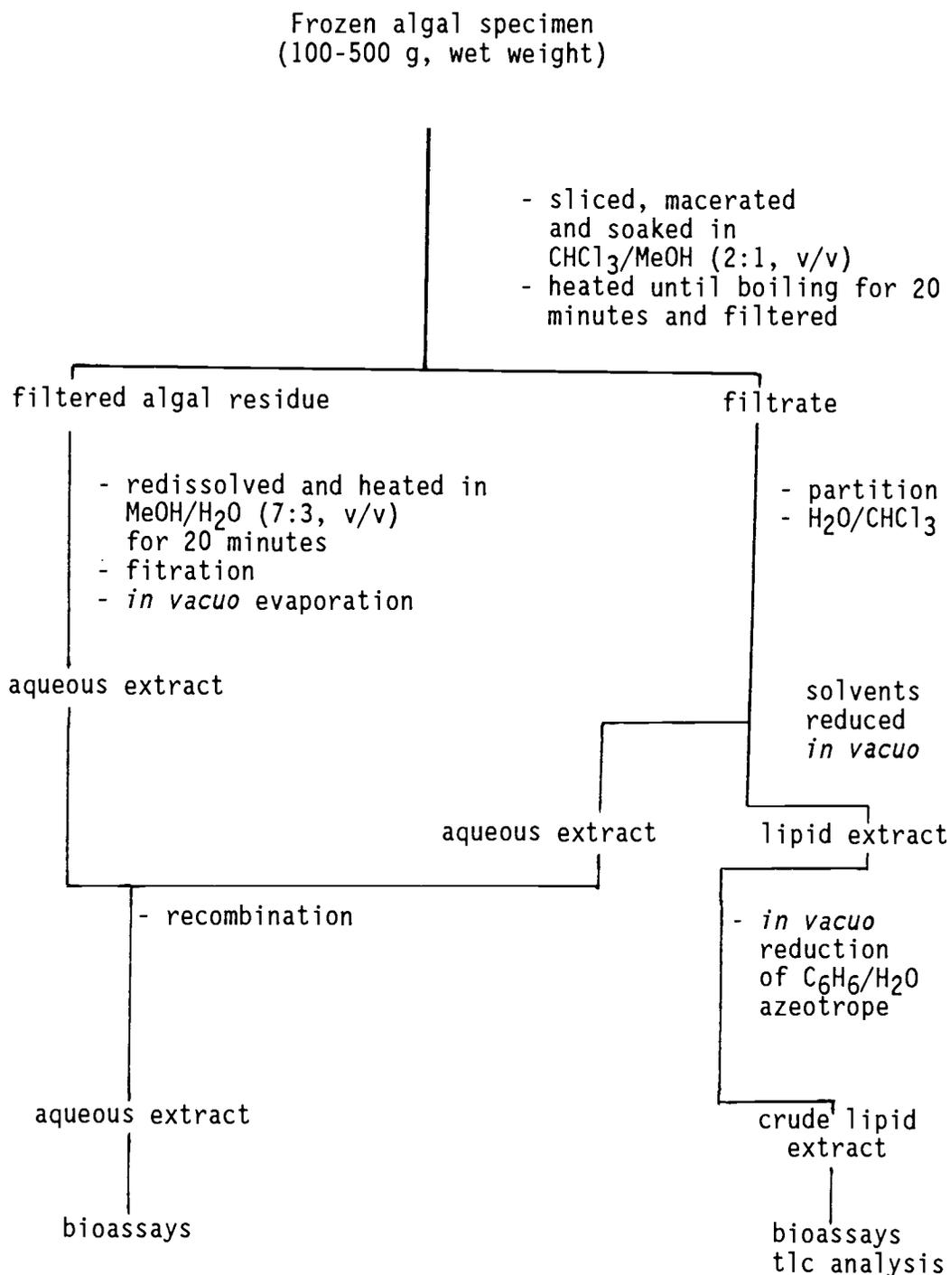
Figure II.1 Generalized extraction scheme.
