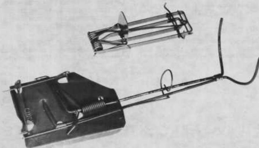
Figure 3.—Victor or Macabee gopher trap (above); cinch trap (below)
