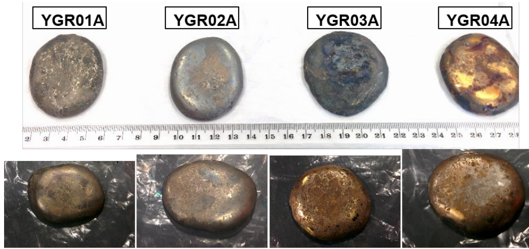
Figure 5.7: As-melted VAR buttons of YGR model alloys, in top row after initial melt in flowing Ar, and in bottom row, after secondary remelting.
