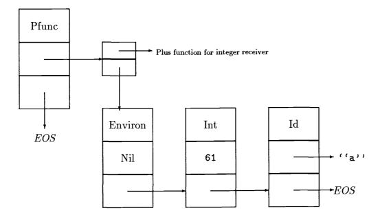
Figure 15: Data Structure for the Primitive Expression 61+a
