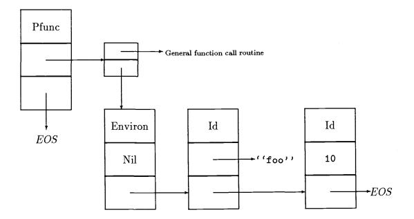
Figure 16: Data Structure for the Function Call foo(10)
