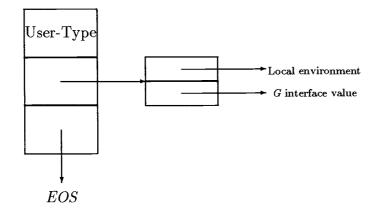
Figure 18: General Representation of an Instance of a User-defined Type
