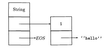
Figure 5: Data Structure that Represents the String "hello"
