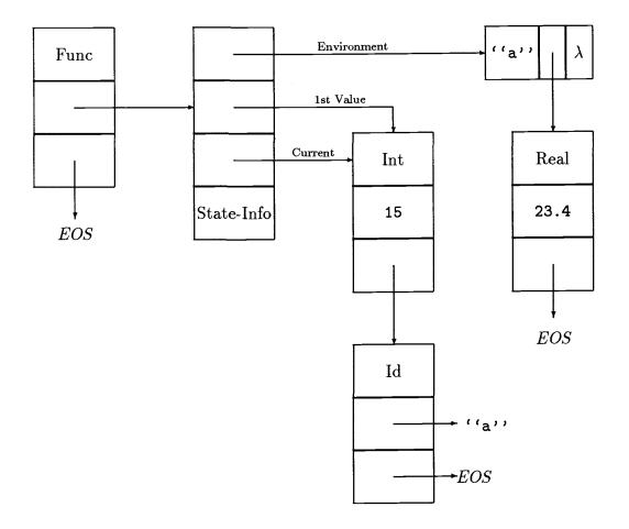
Figure 11: The Function func(a: 23.4)[15, a]
