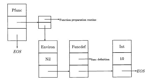
Figure 17: Data Structure for the Function Call func(a)[a](10)
