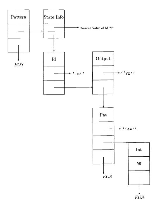
Figure 13: Data Structures for the Value s[?x,<=99]
