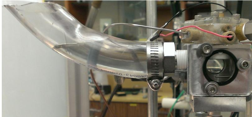
Figure 4.11: Photograph of the liquid-air apparatus showing membrane visibility from the front window allowing high speed camera to focus on the face of the membrane.
