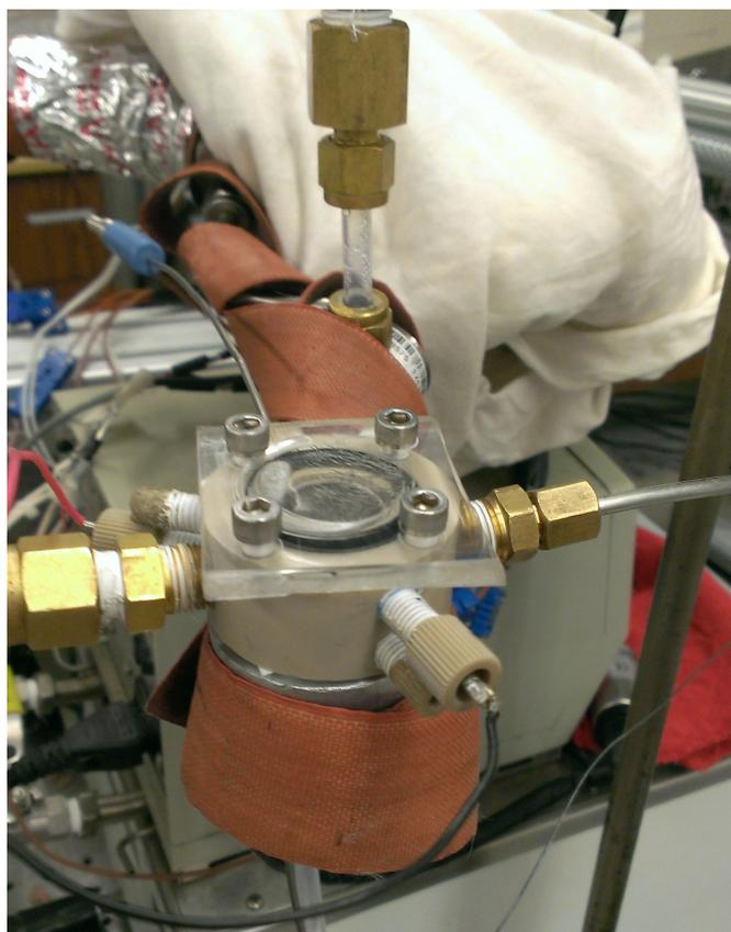
Figure 4.6: Photograph of the superheated vapor apparatus.
