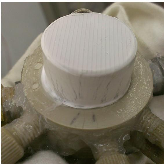
Figure 4.16: Photograph of the extraction chamber after removal from an apparatus to show membrane press fit and vacuum grease on shoulder.
